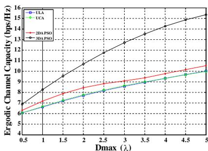
**Figure 10.** The ECC versus  $D_{\max}$  for *Example 3*.
