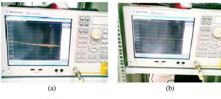
**Figure 7.** Network analyzer for characterization of the EMC of the rice-husk microwave absorber. (a) Before calibration. (b) After two-port calibration.
