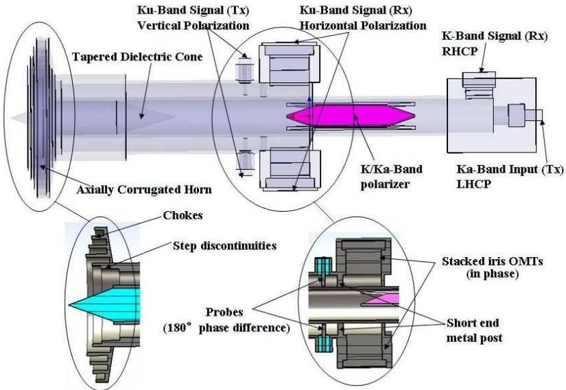
**Figure 3.** Schematic of a compact coaxial-type feed operating at multiple frequencies (Ku/K/Ka-band) and polarizations.
