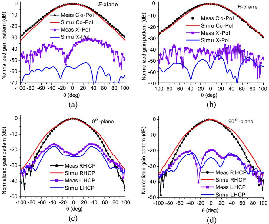
**Figure 5.** Comparison of the simulated and measured gain patterns of the multiband feed at Ku/K-band, (a) 12.5 GHz at  $E$ -plane, (b) 12.5 GHz at  $H$ -plane, (c) 20.5 GHz at  $0^\circ$  cut plane, (d) 20.5 GHz at  $90^\circ$  cut plane.
