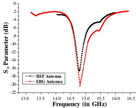
**Figure 6.** S11-parameter versus frequency (in GHz) obtained by measurement for reference antenna and dummy EBG pattern antenna for feedline position 1.0 mm measured from the bottom of the twin patch.
