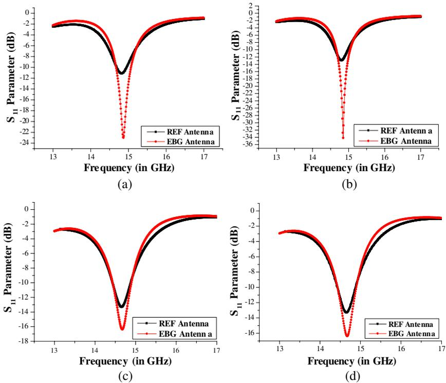
**Figure 4.**  $S_{11}$ -parameter comparison of reference antenna with dummy EBG pattern antennas for 4 different cases (4 feed positions) versus frequency (in GHz). Feedline positions of (a) 1.0 mm, (b) 1.1 mm, (c) 4.05 mm, and (d) 4.1 mm all measured, respectively, from bottom of patch are considered.
