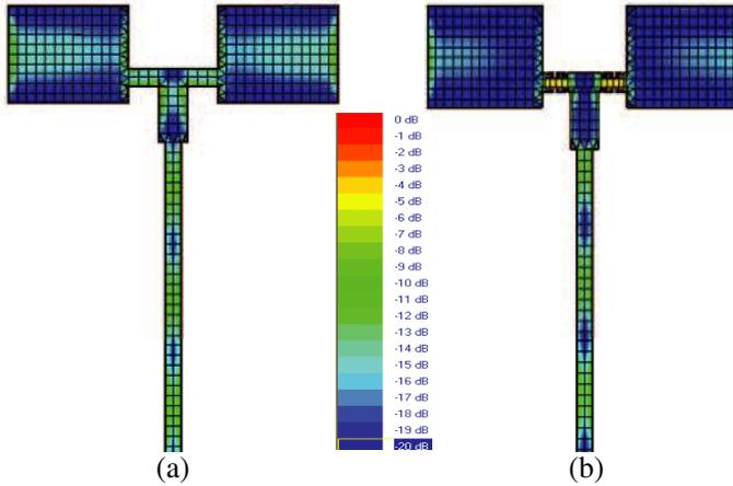
**Figure 7.** Current distribution for reference antenna and dummy EBG pattern antenna when feedline is at a distance of 1.0 mm measured from bottom of twin patch. (a) Current distribution for reference antenna and (b) current distribution for dummy EBG pattern antenna.
