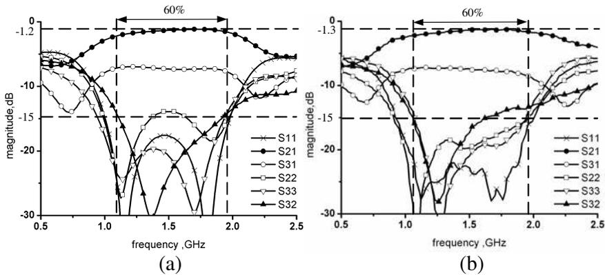
**Figure 10.** Simulated and measured results of proposed 4:1 power divider. (a) Simulated results. (b) Measured results.
