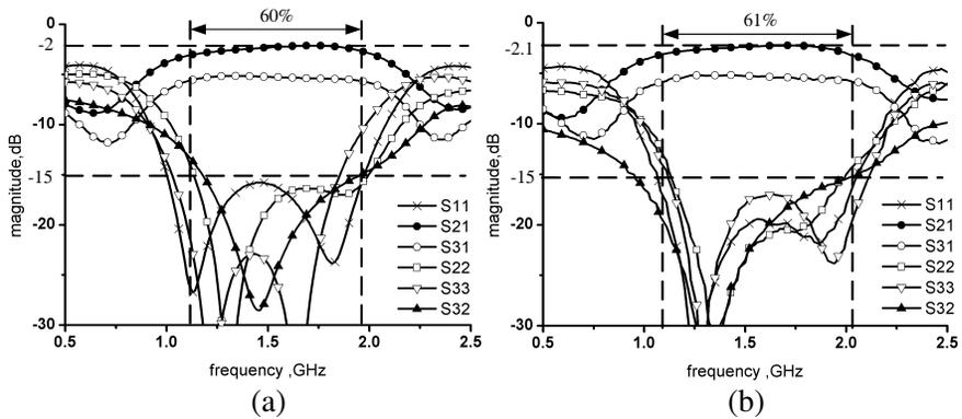
**Figure 8.** Simulated and measured results of proposed 2:1 power divider. (a) Simulated results. (b) Measured results.
