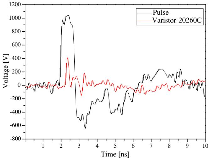
**Figure 11.** The original EMP signal and the treated signal by Varistor (20260C).
