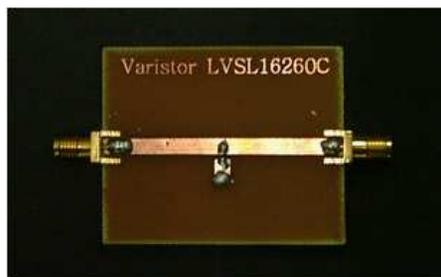
**Figure 6.** PCB mounted varistor.
