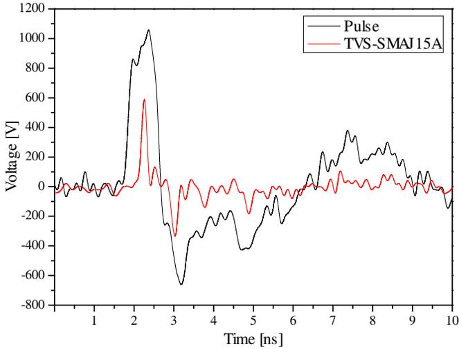
**Figure 8.** The original EMP signal and the treated signal by TVS (SMAJ15A).
