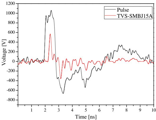
**Figure 9.** The original EMP signal and the treated signal by TVS (SMBJ15A).
