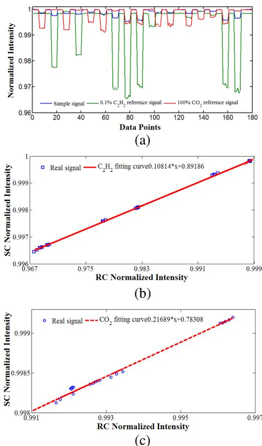
**Figure 6.** (a) Absorption signals in three gas cells; (b) C<sub>2</sub>H<sub>2</sub> concentration in sample versus reference cells and the best linear fit of them; (c) CO<sub>2</sub> concentration in sample versus reference cells and the best linear fit of them.
