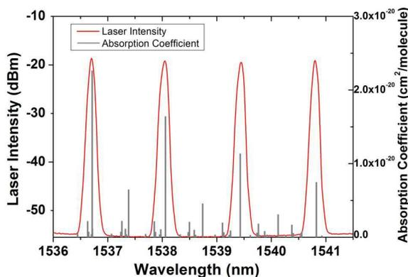
**Figure 2.** The spectrum of 10% power multi-wavelength fiber laser (red line) detected by an optical spectrum analyzer (OSA) before the experiment. Absorption coefficient of  $C_2H_2$  (gray line, calculated with HITRAN 2004) is also shown from 1536 nm to 1541 nm.
