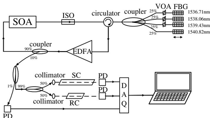
**Figure 1.** The schematic diagram of our multi-wavelength fiber laser-based COSPEC. SOA: semiconductor optical amplifier; ISO: optical isolator; VOA: variable optical attenuator; FBG: fiber Bragg grating; EDFA: erbium-doped fiber amplifier; SC: sample cell; RC: reference cell; PD: photodetector; DAQ: data acquisition card.
