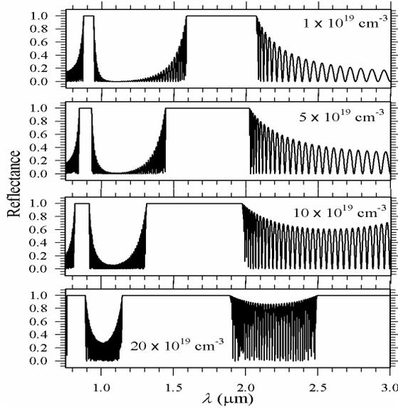
**Figure 4.** The calculated wavelength-dependent reflectance at four different doping concentrations at  $\Lambda = 0.73 \mu\text{m}$ ,  $f = 1/2$ , and  $N_p = 50$ . Two-gap structure is seen for  $N = 1 \times 10^{19}$ ,  $5 \times 10^{19}$ , and  $10 \times 10^{19} \text{ cm}^{-3}$ , but three gaps are obtained at  $20 \times 10^{19} \text{ cm}^{-3}$ .
