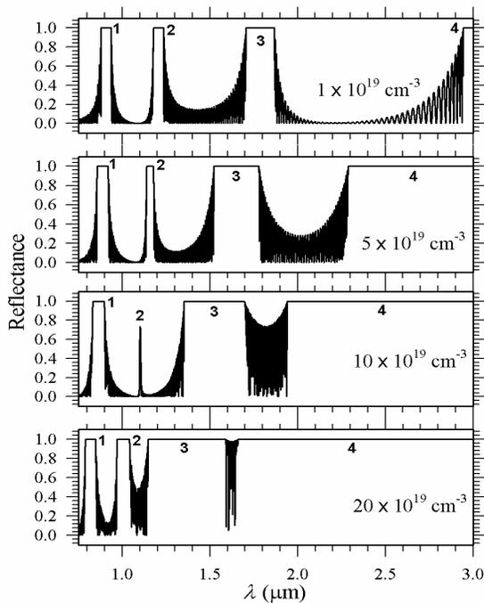
**Figure 6.** The calculated wavelength-dependent reflectance at four different doping concentrations at  $\Lambda = 1.46 \mu\text{m}$ ,  $f = 1/2$  and  $N_p = 50$ . There are four PBGs in the near IR.
