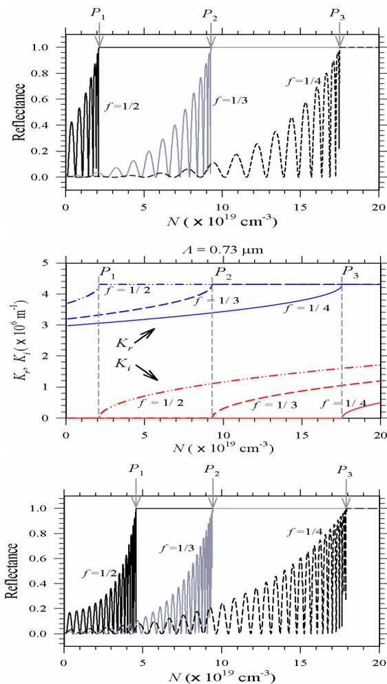
**Figure 3.** The calculated reflectance as a function of the doping concentration for the spatial periodicity  $\Lambda = 0.73 \mu\text{m}$  (upper panel) and  $1.46 \mu\text{m}$  (lower panel) at a fixed wavelength of  $1.54 \mu\text{m}$ . Here,  $N_p = 50$  is used.
