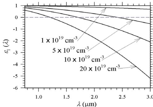
**Figure 2.** The relative permittivity of  $n$ -Si versus wavelength for different doping impurity concentrations of  $N = 1 \times 10^{19}, 5 \times 10^{19}, 10 \times 10^{19}$ , and  $20 \times 10^{19} \text{ cm}^{-3}$  in the case of zero damping frequencies  $\gamma_e = \gamma_h = 0$ .
