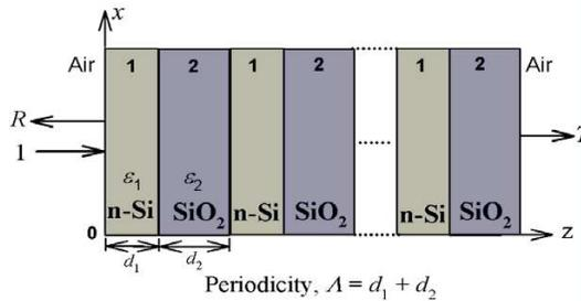
**Figure 1.** A one-dimensional  $n$ -Si/SiO<sub>2</sub> photonic crystal, in which doped  $n$ -type semiconductor  $n$ -Si with thickness  $d_1$  occupies the region 1 and the dielectric SiO<sub>2</sub> with thickness  $d_2$  is in the layer 2, respectively. The spatial periodicity is denoted by  $\Lambda = d_1 + d_2$ . The optical wave with a unit power is launched normally at the plane boundary of  $z = 0$ . The reflectance and transmittance are denoted by  $R$  and  $T$ , respectively.
