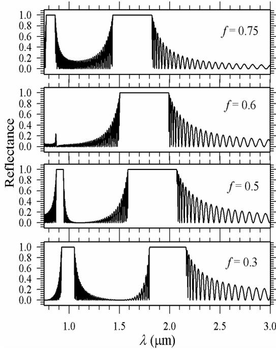
**Figure 7.** The calculated wavelength-dependent reflectance at four different filling factors of  $f = 0.75, 0.6, 0.5,$  and  $0.3$ . Here, at  $\Lambda = 0.73 \mu\text{m}$ ,  $N = 1 \times 10^{19} \text{cm}^{-3}$  and  $N_p = 50$ .
