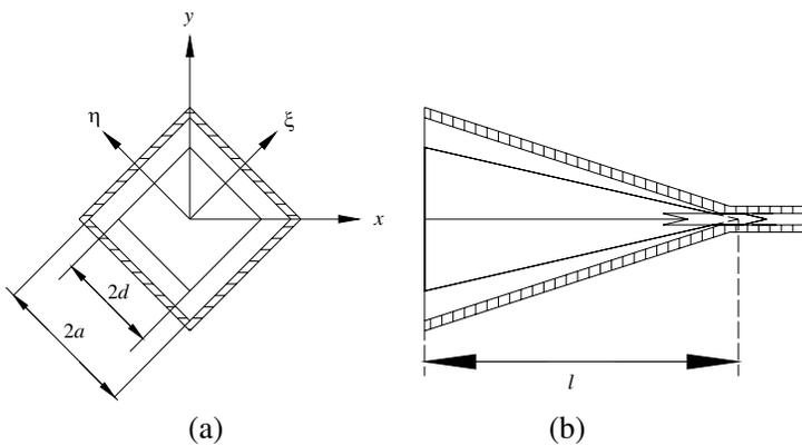
**Figure 2.** The geometry of the dielectric pyramid loaded diagonal horn. (a) Front view of the geometry with the coordinate frame definition. (b) Side view of the dielectric pyramid with the metal diagonal horn longitudinally cut.
