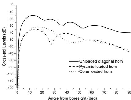
**Figure 13.** The cross-polarized *D*-plane radiation patterns.
