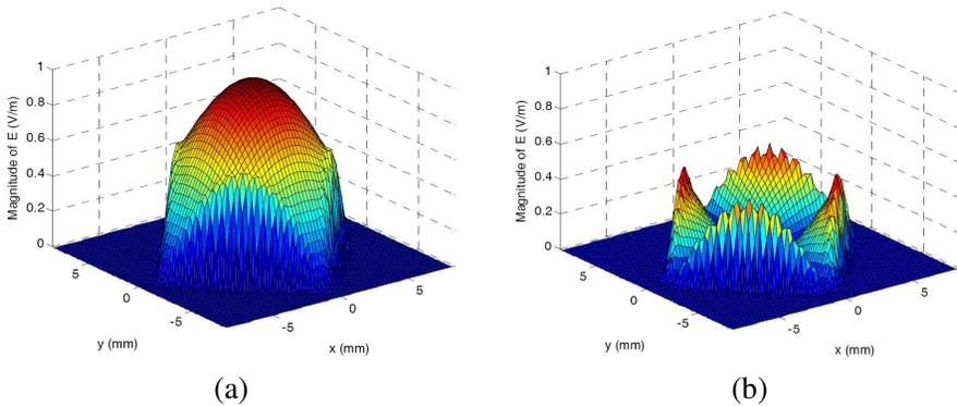
**Figure 6.** The magnitude of the co-polarized and cross-polarized field components at the aperture of a single diagonal horn. (a) Co-polarized component. (b) Cross-polarized component, which is quite large especially at the four edges.
