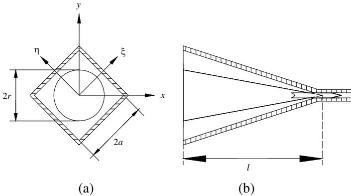
**Figure 8.** The geometry of the dielectric cone loaded diagonal horn. (a) Front view of the geometry with the coordinate frame definition. (b) Side view of the dielectric cone with the metal diagonal horn longitudinally cut.
