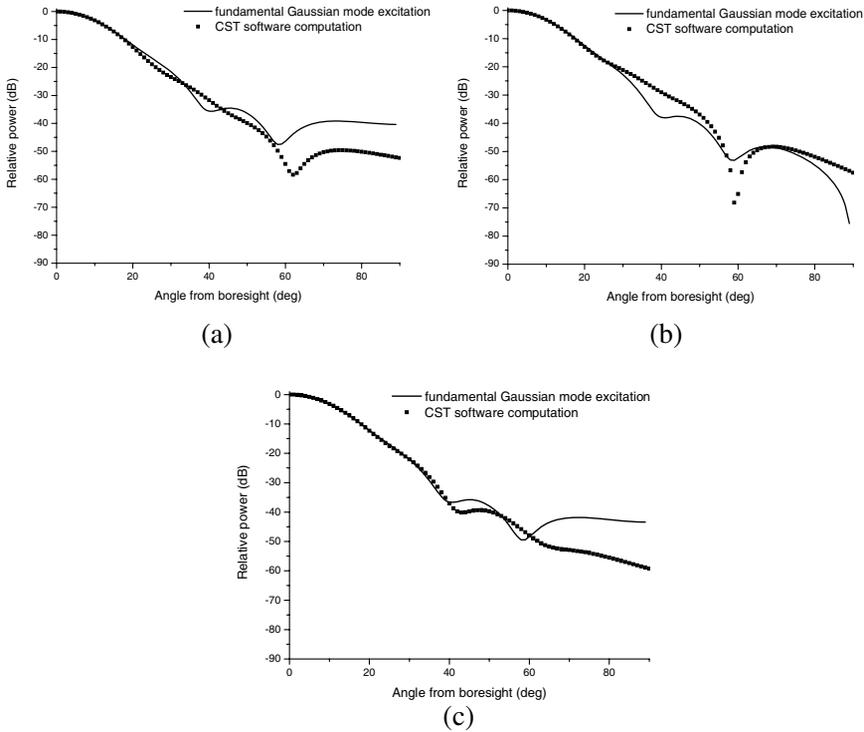
**Figure 12.** The far field prediction of the dielectric cone loaded diagonal horn at 150 GHz. (a)  $E$ -plane, (b)  $H$ -plane, and (c)  $D$ -plane.
