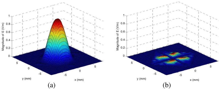
**Figure 9.** The magnitude of co-polarized and cross-polarized field components at the aperture of dielectric cone loaded horn. (a) Co-polarized component, with good axially symmetrical performance and perfect Gaussian distribution. (b) Extremely low cross-polarized component.
