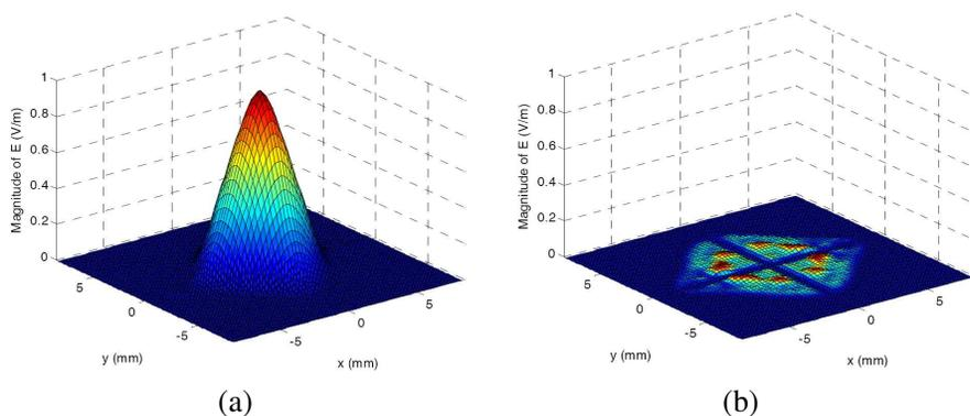
**Figure 5.** The magnitude of the co-polarized and cross-polarized field components at the aperture of the dielectric pyramid loaded horn. (a) Co-polarized component, with good axially symmetrical performance and fine Gaussian distribution. (b) Extremely low cross-polarized component.
