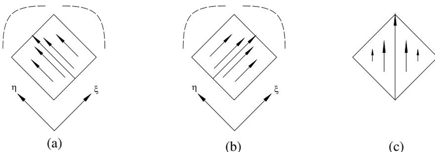
**Figure 4.** The electric field distribution in the aperture of an idealized dielectric diagonal horn. (a)  $E_{11}^{\eta}$  mode with electric field  $\hat{\eta}$ -directed, whose amplitude varies as cosine function with both  $\xi$  and  $\eta$ . (b)  $E_{11}^{\xi}$  mode with electric field  $\hat{\xi}$ -directed, whose amplitude varies as cosine function with both  $\xi$  and  $\eta$ . (c) The superposition of the two modes with equal amplitude and zero phase difference.
