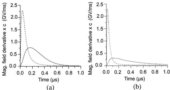
**Figure 4.** Magnetic field time derivative (multiplied by the speed of light) at ground level at 1 km from the lightning channel. The solid line shows the field over finitely conducting ground and the dotted line shows the corresponding one over perfectly conducting ground. (a)  $s = 0.001$  S/m and (b)  $s = 0.0001$  S/m. The relative dielectric constant of ground has been taken as 5. (adopted from [27] and the clarity of the diagram has been improved).
