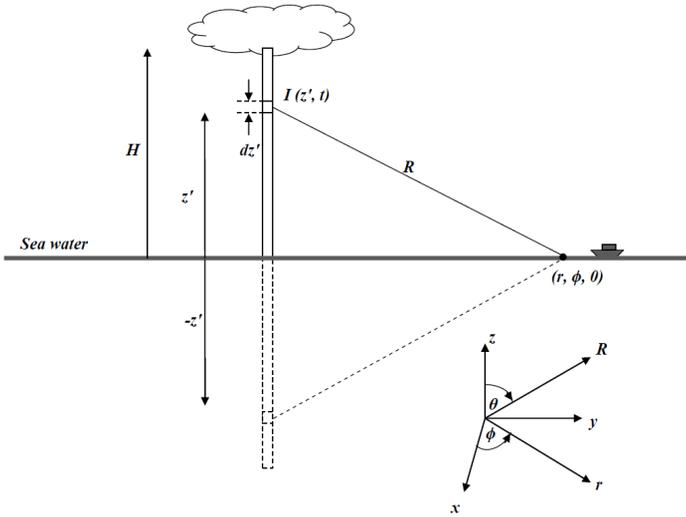
**Figure 2.** Geometrical parameters corresponding to the equations that calculate electric and magnetic fields at ground level over perfectly conducting plane (such as sea water).
