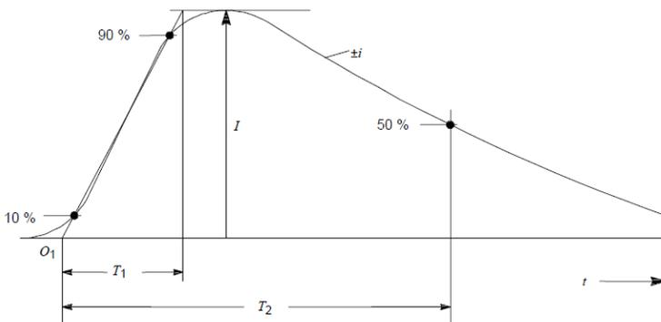
**Figure 1.** The profile of the test waveform specified in many standards to represent lightning impulse current. The time  $T_1$  is approximately equal to the rise time of the waveform. The time  $T_2$  gives the half peak width of the waveform. A certain combination of  $T_1$  and  $T_2$  specifies a given test waveform (adopted from [14]).
