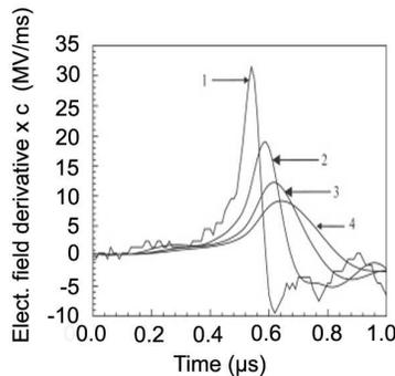
**Figure 3.** Variation of electric field derivative of a first return stroke as it propagates over ground of conductivity 0.001 S/m: (1) Undistorted field (i.e., infinite conductivity), (2) after propagating 1 km, (3) after propagating 4 km and (4) after propagating 8 km (adopted from [18] and the clarity of the diagram has been improved).
