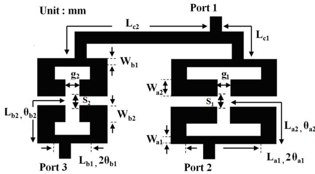
**Figure 1.** Schematic of the proposed diplexer. The right part is the BPF section for GPS application and the left part is the BPF section for WLAN application. The input line with branch structure is tapped to two BPFs to provide the input power and the impedance matching.
