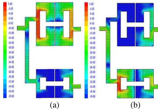
**Figure 9.** Simulated current distribution and coupling paths oscillating of the diplexer at the centre frequency at (a) 1.575 GHz and (b) 2.4 GHz.
