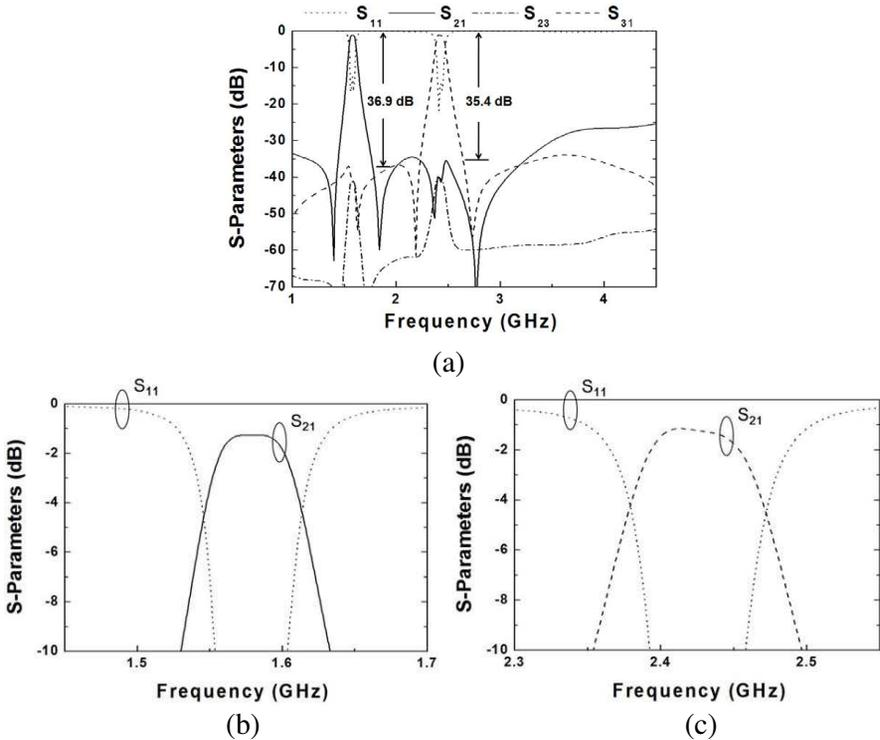
**Figure 8.** (a) Simulated frequency responses of the proposed diplexer with the impedance matching, and the simulated passbands at (b) 1.575 GHz and (c) 2.43 GHz in detail.
