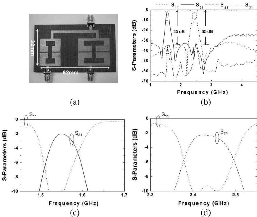
**Figure 10.** (a) Photograph and (b) measured frequency responses of the fabricated diplexer and the measured passbands at (c) 1.575 GHz and (d) 2.43 GHz in detail.
