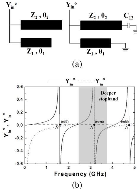
**Figure 4.** (a) Equivalent circuit for analysing even mode ( $Y_{in}^e$ ) and odd mode ( $Y_{in}^o$ ) of the modified SIR and (b) the calculated values of  $Y_{in}^e$  and  $Y_{in}^o$  as  $Z_1 = 54 \Omega$ ,  $Z_2 = 28.6 \Omega$ ,  $L_{a1} = 17.63 \text{ mm}$ ,  $L_{a2} = 18.93 \text{ mm}$  for 1.575 GHz.
