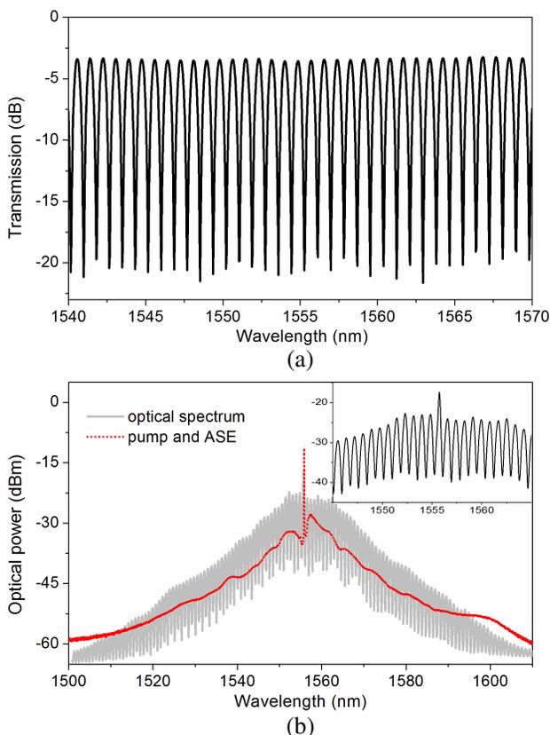
**Figure 2.** (a) Transmission spectrum of the Sagnac loop filter. (b) Spectra of the proposed MW-FOPO (gray solid curve) and the ASE of the FOFA (red dotted curve). Inset shows a local enlargement of the spectrum from 1545 nm to 1565 nm.
