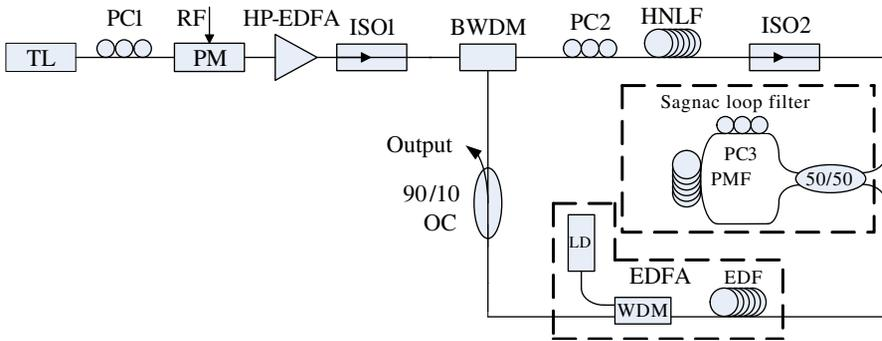
**Figure 1.** Experimental setup of the proposed MW-FOPO. TL: tunable laser; PC: polarization controller; PM: phase modulator; HP-EDFA: high power Erbium-doped fiber amplifier; ISO: isolator; BWDM: broadband wavelength division multiplexer; HNLf: highly nonlinear fiber; OC: optical coupler; PMF: polarization maintained fiber; EDF: Erbium-doped fiber; LD: Laser diode.
