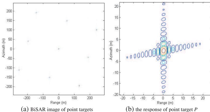
**Figure 6.** Imaging results of proposed PFA for BiSAR.
