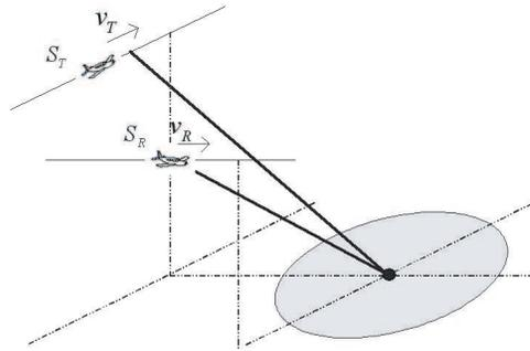
**Figure 5.** The BiSAR illumination geometry for simulation.
