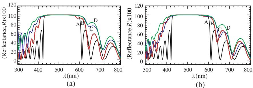
**Figure 5.** Reflectance response as a function of the wavelength at  $N = 11$ . Curve A: The ideal quarter-wavelength stack; Curve B:  $D = 0.1$ , single disorder for  $\text{MgF}_2$ ; Curve C:  $D = 0.1$ , single disorder for  $\text{ZnS}$ ; Curve D:  $D = 0.1$  double disorder. Here (a) is for the disorder made by Eq. (1) and (b) is by Eq. (3).
