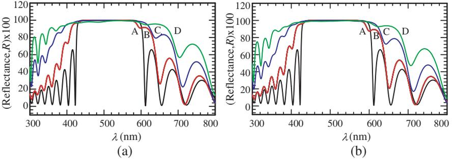
**Figure 4.** Reflectance response as a function of the wavelength for the ideal (A) and double disorder dielectric mirrors (B, C, and D). The double disorder is designed on both  $\text{ZnS}$  and  $\text{MgF}_2$  layers with equal  $D = 0.05$  (B),  $0.1$  (C), and  $0.15$  (D) and  $N = 11$ . Here (a) is for the disorder made by Eq. (1) and (b) is by Eq. (3).
