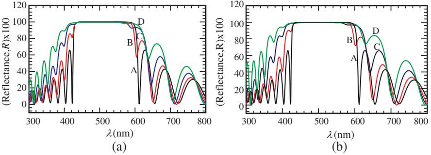
**Figure 3.** Reflectance response as a function of the wavelength for the ideal (A) and disorder dielectric mirrors (B, C, and D). The single disorder is designed on  $\text{MgF}_2$  layers with  $D = 0.05$  (B),  $0.1$  (C), and  $0.15$  (D) and  $N = 11$ . Here (a) is for the disorder made by Eq. (1) and (b) is by Eq. (3).
