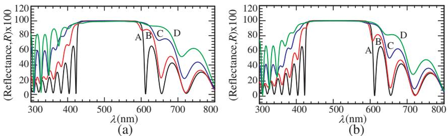
**Figure 2.** Reflectance response as a function of the wavelength for the ideal (A) and disorder dielectric mirrors (B, C, and D). The single disorder is designed on ZnS layers with  $D = 0.05$  (B),  $0.1$  (C), and  $0.15$  (D) and  $N = 11$ . Here (a) is for the disorder made by Eq. (1) and (b) is by Eq. (3).
