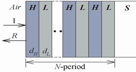
**Figure 1.** An ideal dielectric mirror made of high/low-index quarter-wavelength layers  $H$  and  $L$ , i.e.,  $n_H d_H = n_L d_L = \lambda_0/4$ , where  $\lambda_0$  is the design wavelength.
