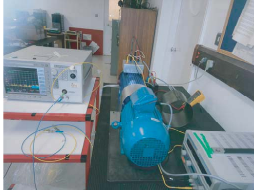
Figure 3. Experimental set up showing a circular metal plate with the same diameter as a 2.2 kW induction machine having fibre bonded on to it at multiple points and connected to the OSA and LabView.
