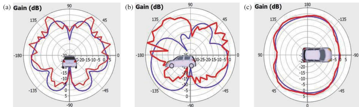
**FIGURE 10.** Radiation patterns analysis at 5.8 GHz for various planes, (a)  $XY$ -plane, (b)  $YZ$ -plane, (c)  $ZX$ -plane [Red colour indicates measurement results and Blue colour indicates simulation results].
