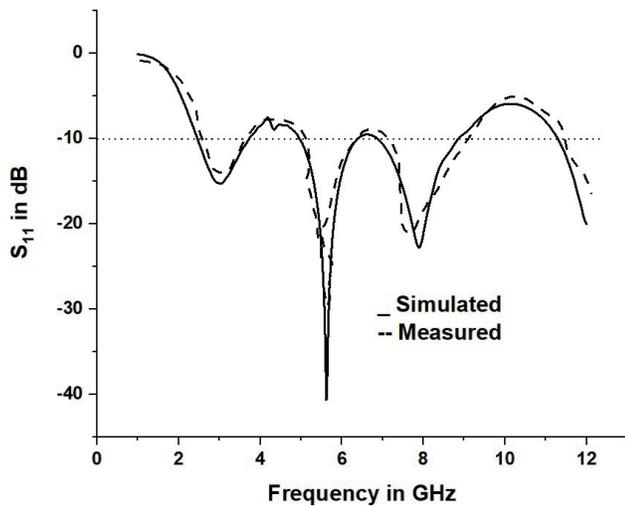
FIGURE 4.  $S_{11}$  parameter of proposed antenna.
