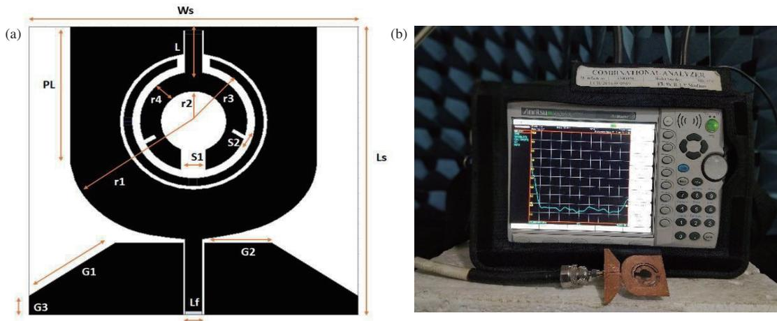
FIGURE 2. Proposed antenna. (a) Design. (b) Prototype measurement.
