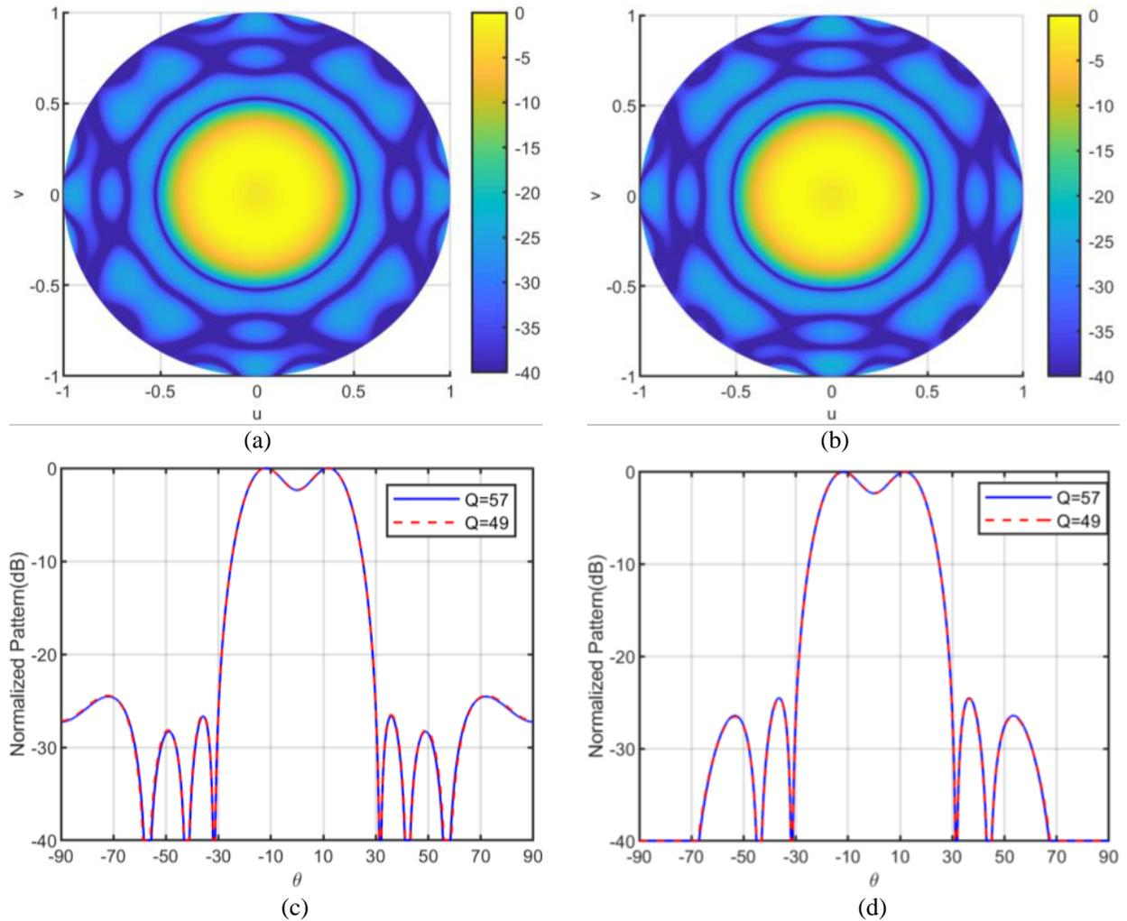
**Figure 10.** Comparison of the reconstructed flat-top patterns. (a) The sparse array with 57 elements in [27], (b) the sparse array with 49 elements herein, (c)  $\varphi = 0^\circ$  plane, (d)  $\varphi = 45^\circ$ .
