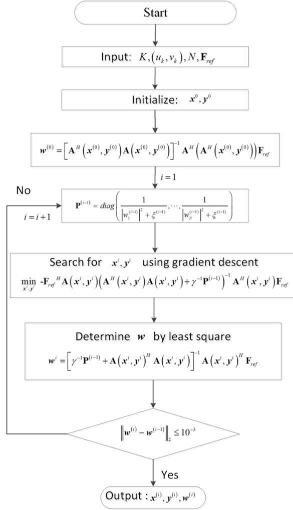
Figure 1. The flowchart of the synthesis process.
