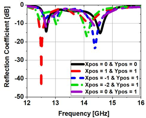
Figure 5. Simulated reflection coefficients for different  $X$  pos &  $Y$  pos values.
