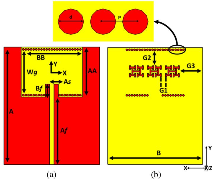
**Figure 2.** Schematic diagram of the proposed antenna. (a) Top view. (b) Bottom view.
