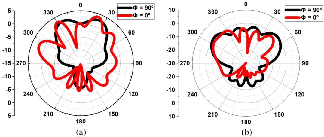
Figure 8. Simulated radiation patterns (a) at 12.67 GHz, (d) at 14.56 GHz.
