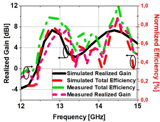
Figure 7. Simulated and measured realized gain & antenna efficiency.
