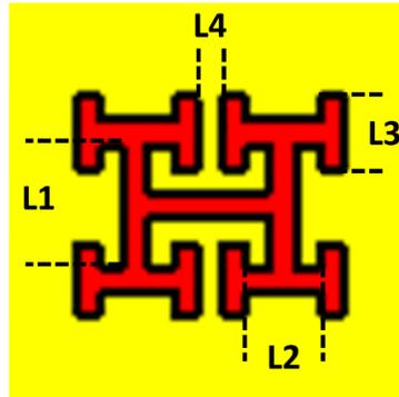
**Figure 1.** The geometry of H-DGS unit cell.
