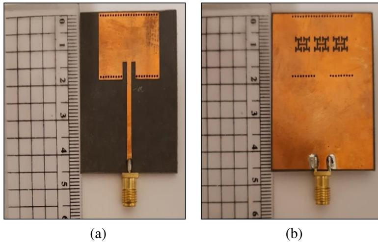
**Figure 3.** Unit cell of the H shaped DGS. (a) Top view. (b) Bottom view.
