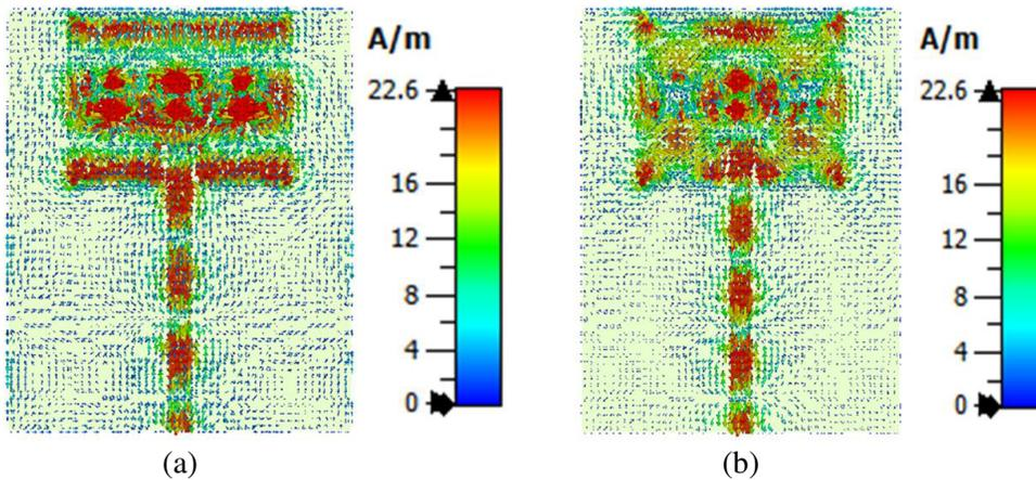
Figure 9. Surface current distribution (a) at 12.67 GHz, (b) at 14.56 GHz.
