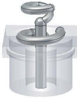
**Figure 3.** Structure of the dual-branch helical antenna.
