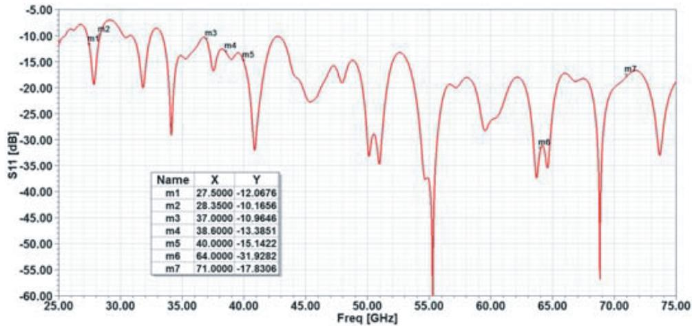
Figure 2. The antenna return loss in free space.
