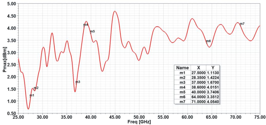
Figure 7. Maximum output power of the antenna.
