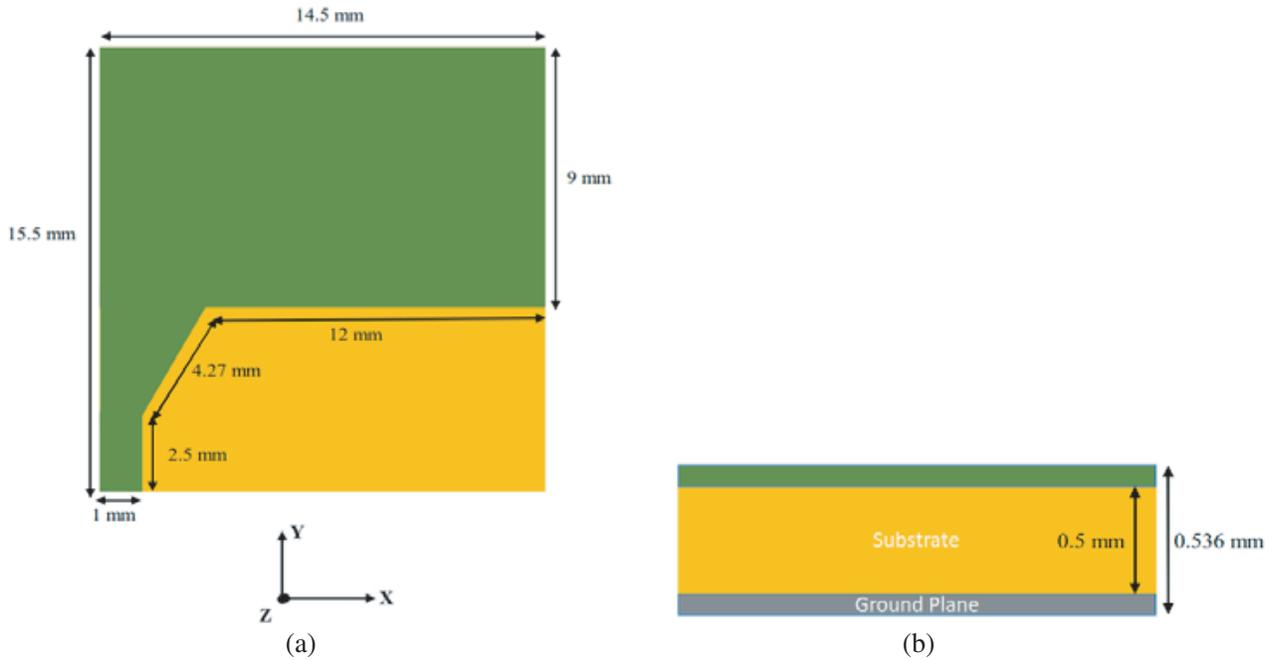
Figure 1. The antenna design configuration, (a) top view, (b) side view.
