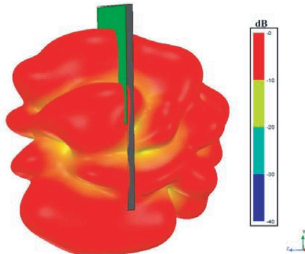
**Figure 6.** 3-D total radiation far-field pattern at 38 GHz.
