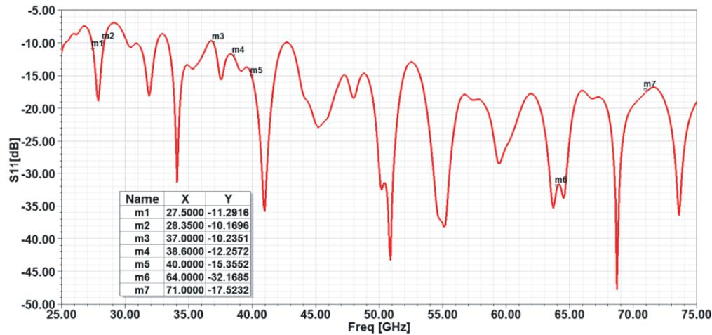
**Figure 5.** Antenna return loss at distance of 10 mm from head.
