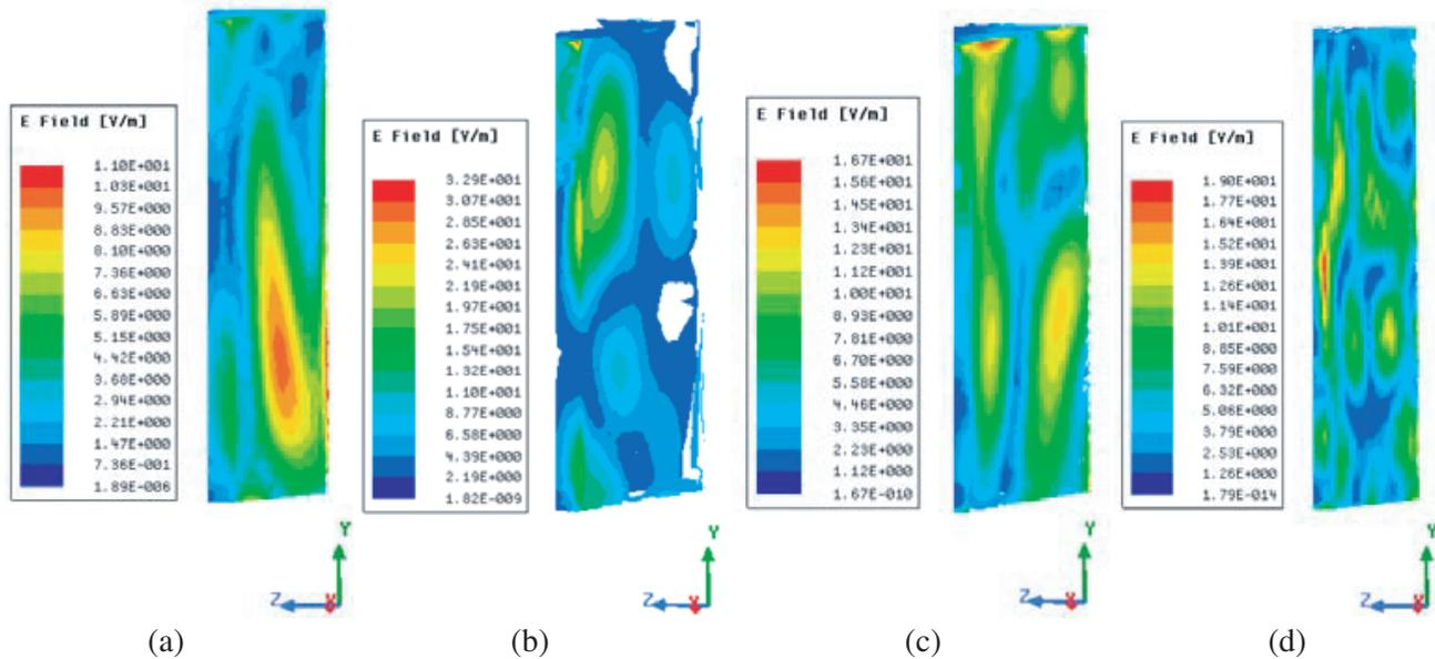
Figure 8. Electric field intensity on the surface of tissue at (a) 28 GHz, (b) 38 GHz, (c) 40 GHz, and (d) 67 GHz.
