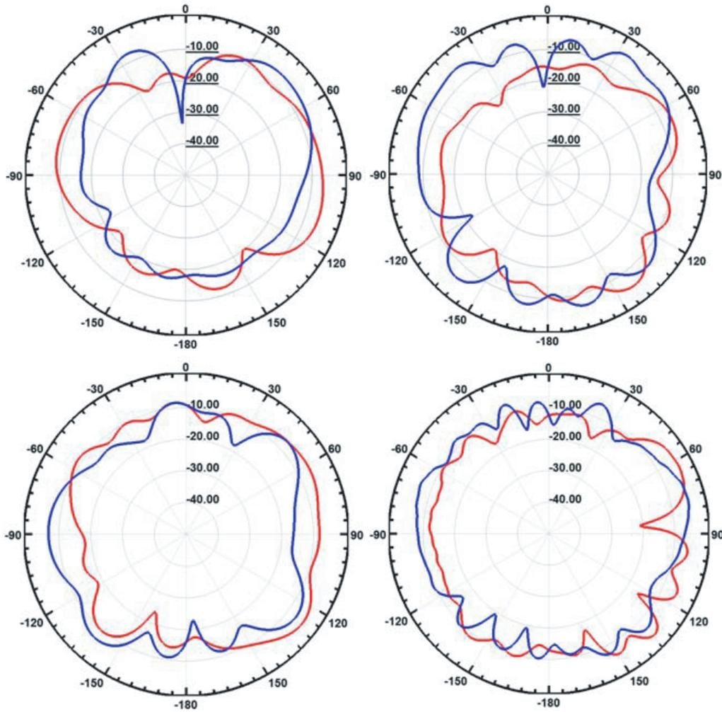
**Figure 3.** Radiation patterns at  $\varphi = 0^\circ$  and  $\varphi = 90^\circ$  at 28 GHz, 38 GHz, 40 GHz, and 67 GHz.
