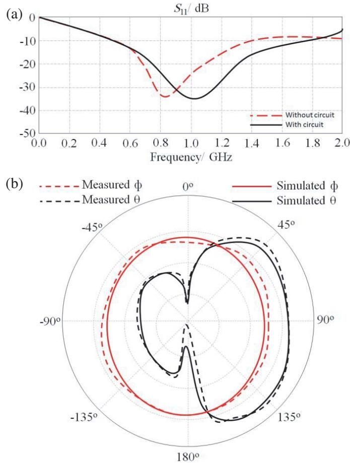
**Figure 10.**  $S_{11}$  measurements before and after attaching the RF circuit converter: (a)  $S_{11}$  spectra and (b) radiation patterns.
