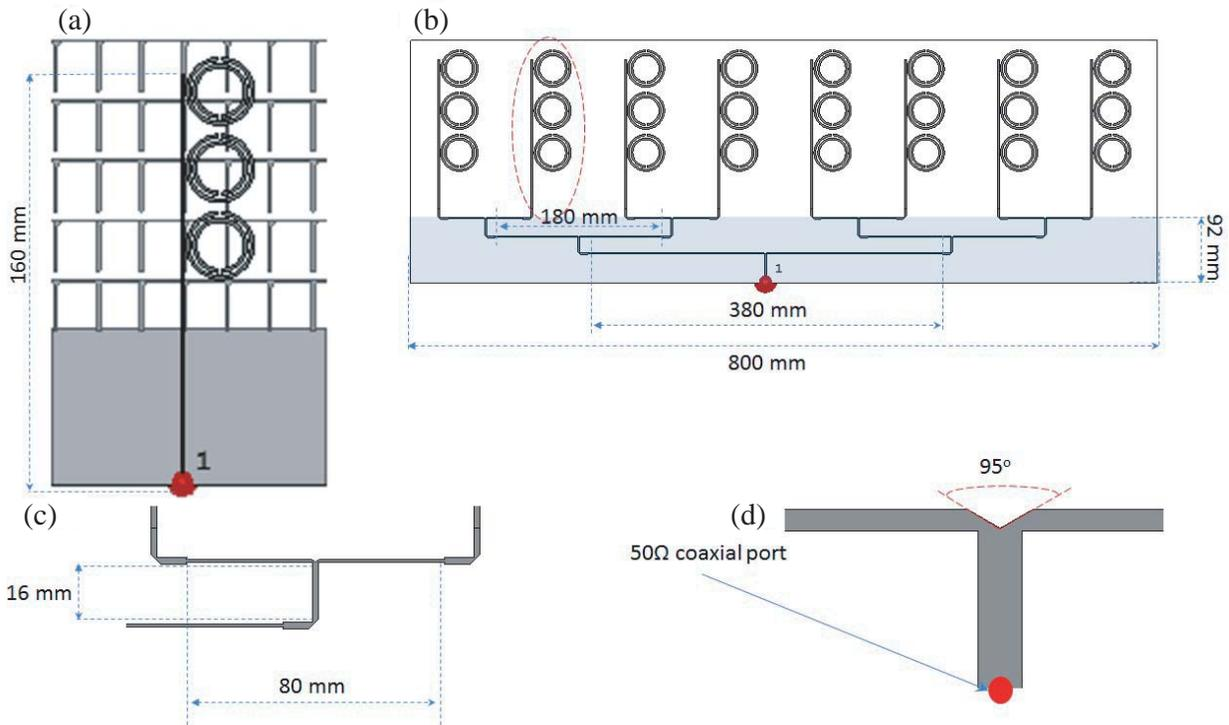
**Figure 4.** The proposed antenna structure; (a) single element, (b) array, (c) transmission line, and (d) discrete coaxial probe fee.
