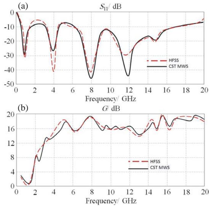
**Figure 6.** The numerical simulation results of the antenna array: (a)  $S_{11}$  and (b) gain spectra.
