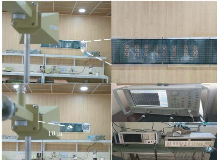
**Figure 8.** The measurement setup including the horn antenna, the proposed antenna array and the VNA pictures.
