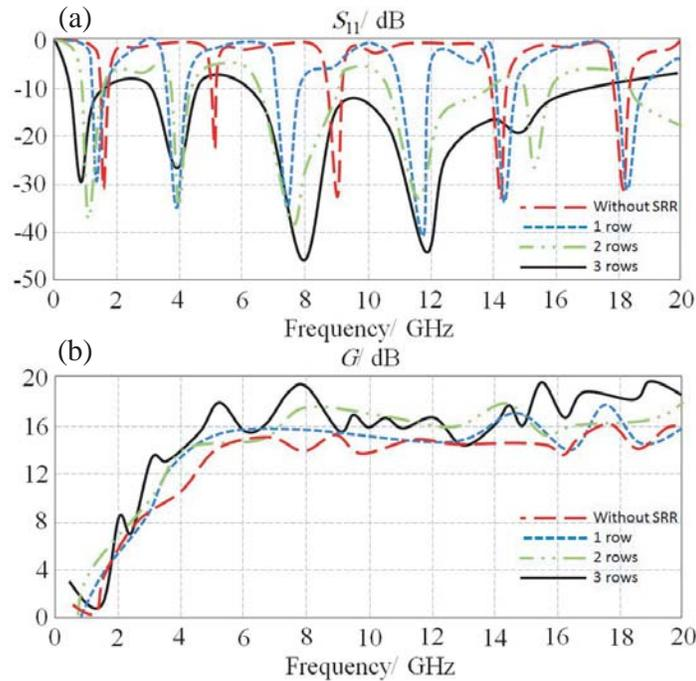
**Figure 5.** The simulated  $S_{11}$  and gain spectra of the proposed antenna with different number of the SRR rows.
