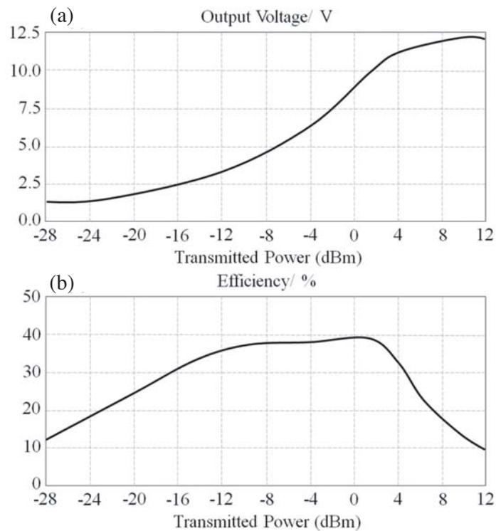
**Figure 9.** The measured results: (a) Output voltage and (b) efficiency.
