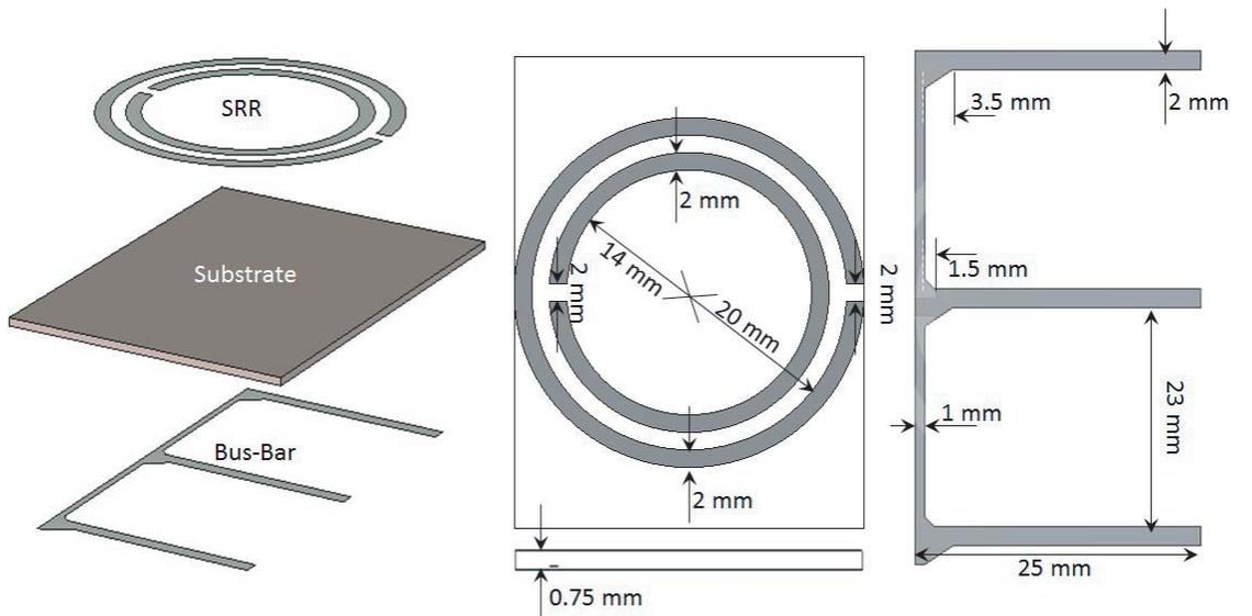
**Figure 1.** The geometrical details of the proposed SRR.
