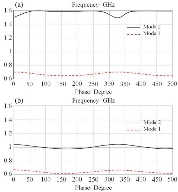
**Figure 3.** The evaluated dispersion diagram of the proposed SRR: (a) Without bus-bar and (b) with bus-bar.
