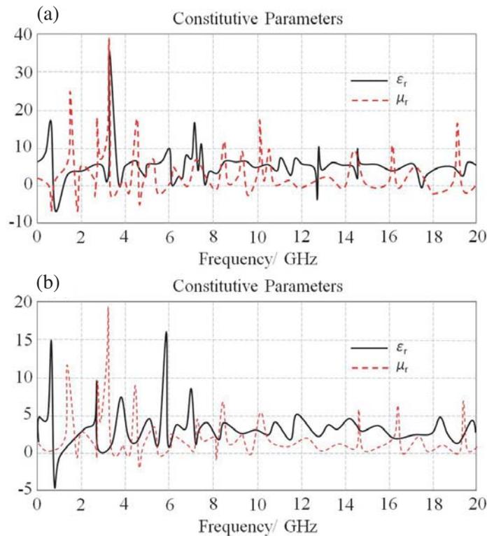
**Figure 2.** The evaluated  $\epsilon_r$  and  $\mu_r$  of the proposed SRR: (a) Without bus-bar and (b) with bus-bar.
