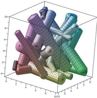
**Figure 1.** (Color on line.) The 3D cluster of disordered cylindrical nanotubes having normal distribution on height  $h$  and radius  $r$ . It is considered that the parameters of nanotubes are distributed normally, see Eq. (1).
