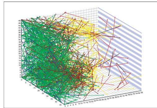
**Figure 2.** (Color on line.) Details of the spatial structure of the normal distribution of percolating cylinders with  $\mu_h = 20, \sigma_h = 2, \mu_r = 0.1, \sigma_r = 0.025$  that belong to the infinite cluster slightly above the percolation threshold  $p = 0.1 > p_c = 0.05$ . The grid is  $50 \times 50 \times 60$  is used. Only the cylinders connected to the infinite cluster are shown.
