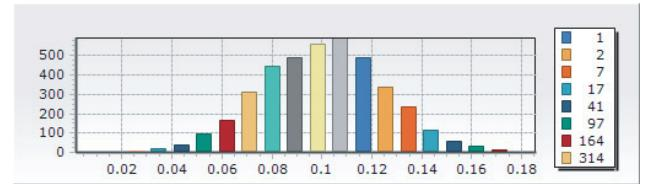
**Figure 4.** (Color on line.) The histogram of normal distribution of the radius  $r$  for cylinders generated for  $\mu_r = 0.01$  and  $\sigma_r = 0.025$  (with  $r_{\max} = 0.18, r_{\min} = 0.01$ ).
