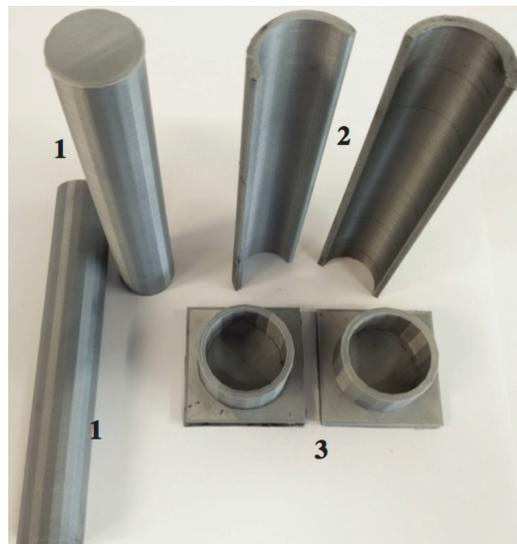
**Figure 5.** Cylindrical plugs (1) used to make cylindrical cavities in the brain layer and cylindrical phantom plug mould equipment (2, 3). To create a plug, the phantom material is packed into the two halves (2), which are then joined and held together by the supports (3) shown which are placed on the top and bottom of the joined halves until the material sets.
