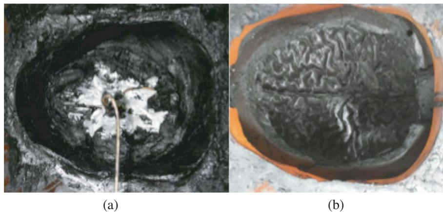
**Figure 4.** (a) External layer poured and laid inside the head counter mould with the brain mould positioned inside, a wire is attached to the brain mould to aid in its removal once the external layer is set. (b) Once set, the brain mould is removed intact to leave the outer layer with an impression of the exterior surface of the brain on its inner side.
