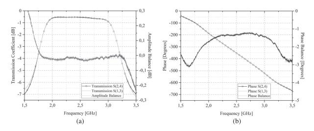
Figure 5. (a) Measured magnitude balance and (b) phase balance between RF ports 1-3 and 2-4.
