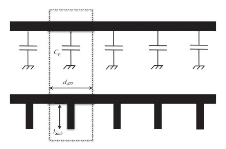
Figure 2. Stub-loaded Artificial Transmission Line (ATL).
