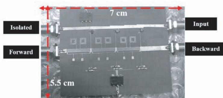
**Figure 3.** Fabricated prototype, of the proposed dual-band DM.
