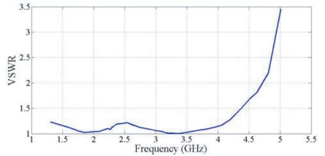
**Figure 5.** The measurement VSWR of the proposed DM.
