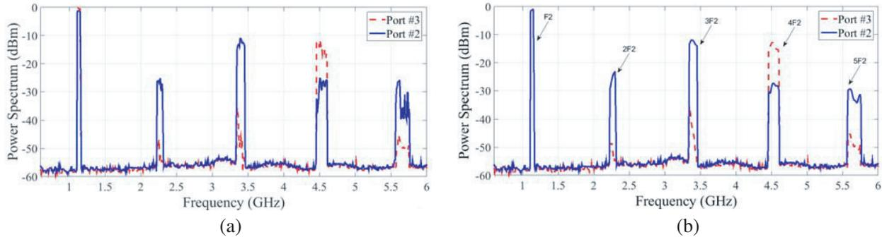
**Figure 7.** Output power spectrum of the proposed dual-band distributed multiplier shown in Fig. 2 at input frequency  $f_2 = 1110 \sim 1160$  MHz. (a) full-wave simulation results. (b) Measurement results.
