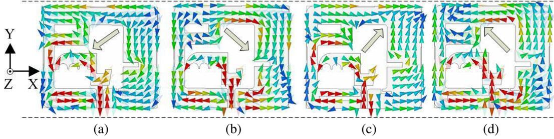
**Figure 2.** Simulated surface vector current distributions of proposed antenna at 4 GHz for four phases. (a)  $0^\circ$ , (b)  $90^\circ$ , (c)  $180^\circ$ , (d)  $270^\circ$ .
