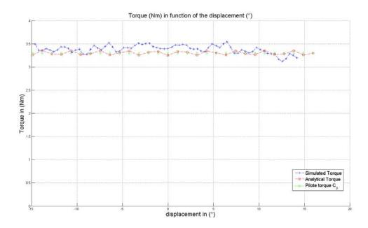
Figure 13. Comparison of the evolution of the simulated and analytical torque in a full range of movement of the DARM which respects the set 1.
