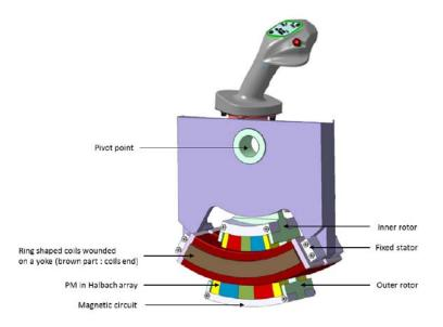
Figure 2. Double airgap rotative machine (DARM).
