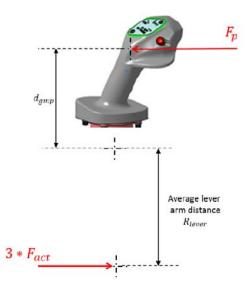
Figure 3. Grip middle point distance and average lever arm distance.
