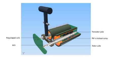
Figure 1. Tubular moving magnet actuator (MMA).
