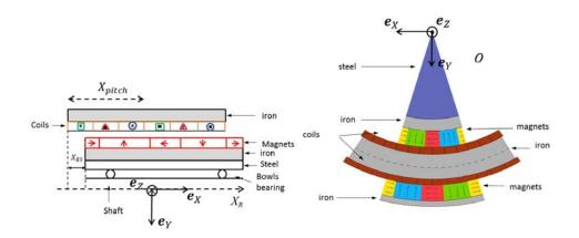
Figure 7. Coordinates systems for both structures.
