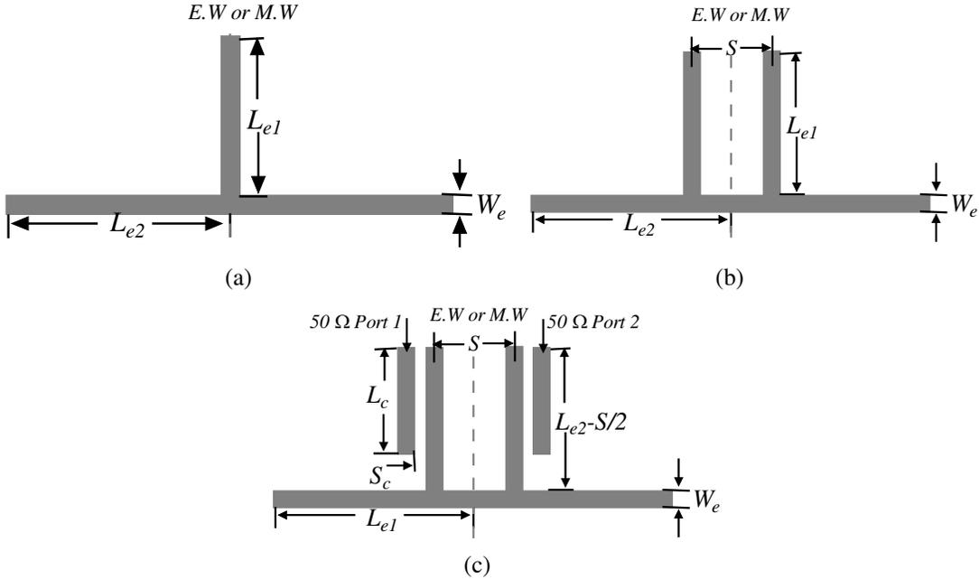
**Figure 1.** (a) Initial dual-mode stub-loaded resonators in [8]. (b), (c) Proposed triple-mode stub-loaded resonators and triple-mode bandpass filters with parallel-coupling feed structures.
