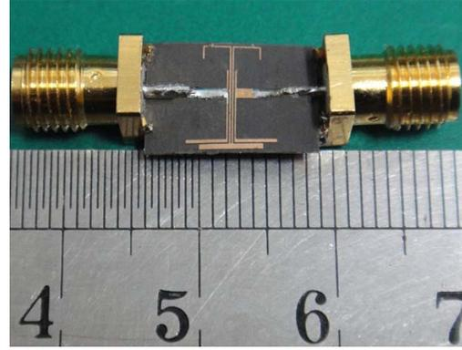
**Figure 4.** Photograph of the fabricated microstrip narrow Ku-band bandpass filter.
