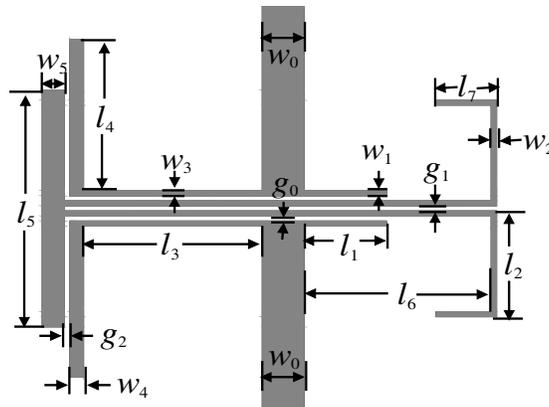
Figure 2. Layout of the proposed microstrip narrow Ku-band bandpass filter.
