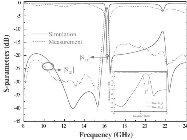
**Figure 3.** Simulated and measured  $S$ -parameters of the proposed microstrip narrow Ku-band bandpass filter.
