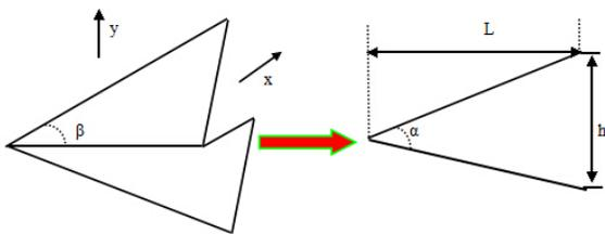
Figure 2. The structure of original TEM horn antenna.
