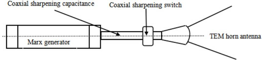
**Figure 1.** The structure of FREMP.
