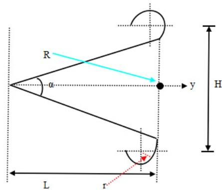
Figure 3. The structure of new TEM horn antenna.
