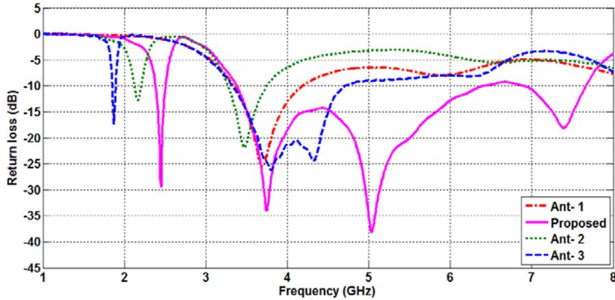
**Figure 3.** Simulated return loss curves of various ACS-fed structures in the design evolution process.
