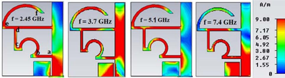
**Figure 4.** Simulated surface current distributions of the antenna at 2.45 GHz, 3.7 GHz, 5.0 GHz and 7.4 GHz.
