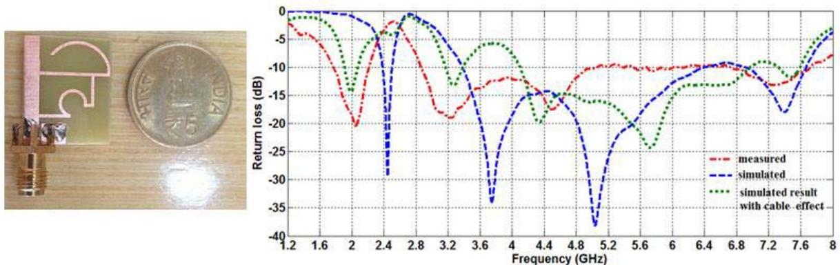
**Figure 6.** Fabricated prototype photograph and its simulated and measured return loss against frequency.
