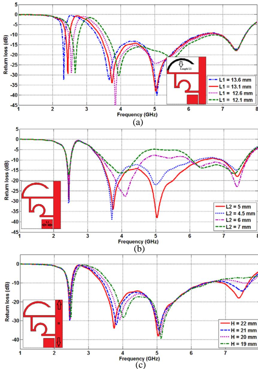
**Figure 5.** (a) Simulated return loss characteristics of the proposed antenna with varied  $L1$ . (b) Simulated return loss characteristics of the proposed antenna with varied  $L2$ . (c) Simulated return loss characteristics of the proposed antenna with varied  $H$ .
