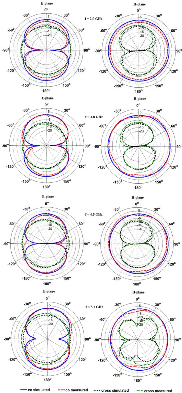
**Figure 7.** Simulated and measured radiation patterns of the proposed ACS-fed dual-band antenna at 2.0 GHz, 3.8 GHz, 4.5 GHz and 5.1 GHz.
