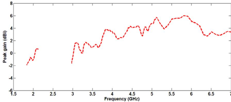
**Figure 8.** Measured peak gain of the proposed ACS-fed dual-band antenna.
