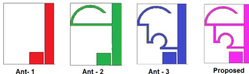
Figure 2. Evolution process of the dual-band monopole antenna.
