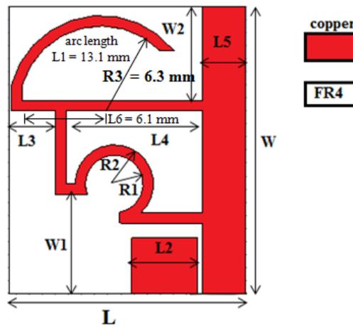
Figure 1. Geometry of the proposed ACS-fed dual-band antenna.
