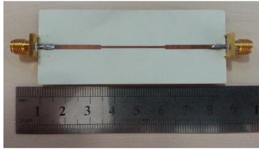
**Figure 9.** Prototype of the step microstrip line.
