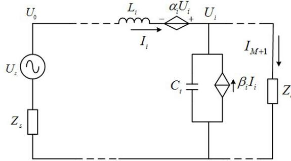
Figure 2. Equivalent circuit of the step microstrip line.
