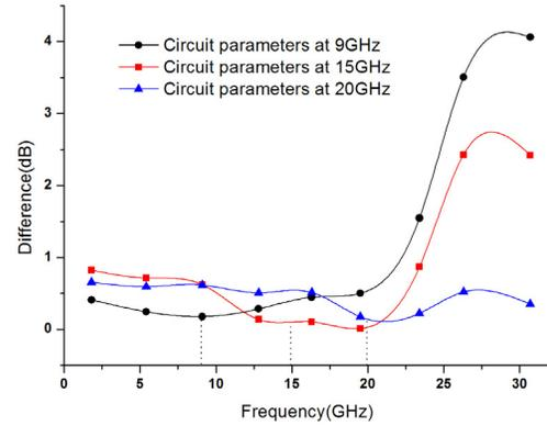
**Figure 8.** Difference between the peaks of  $|S_{11}|$  curve obtained from the circuit parameters and CST.
