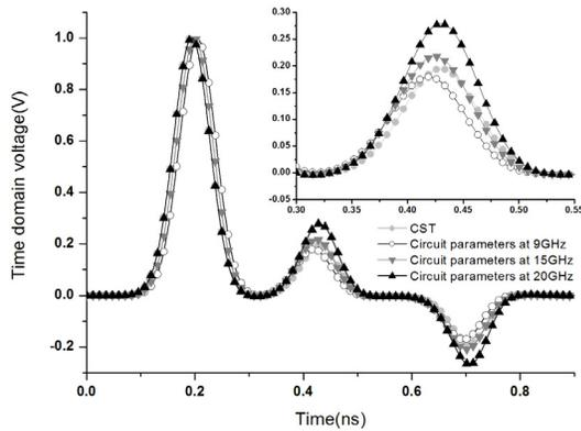
**Figure 5.** Total voltage waveforms at the monitoring point when  $g = 18 \times 10^9 \text{ s}^{-1}$ .
