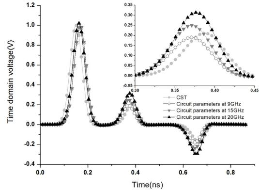
**Figure 6.** Total voltage waveforms at the monitoring point when  $g = 24 \times 10^9 \text{ s}^{-1}$ .
