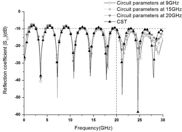
**Figure 7.** Comparison of the reflection coefficient  $|S_{11}|$  obtained from the circuit parameters and CST.
