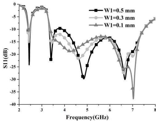
**Figure 4.** Return loss against frequency with different  $W_1$ .
