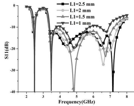
**Figure 7.** Return loss against frequency with different  $L_1$ .
