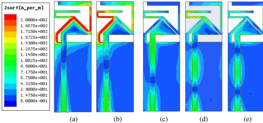
**Figure 8.** Surface current distribution on the proposed antenna at various resonant frequencies: (a) 2.43 GHz, (b) 3.43 GHz, (c) 4.62 GHz, (d) 6.59 GHz, and (e) 7.05 GHz.
