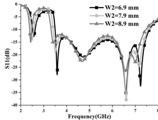
**Figure 5.** Return loss against frequency with different  $W_2$ .
