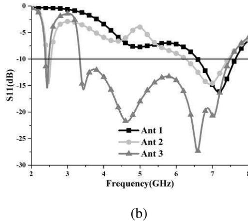
Figure 3. Comparison of simulated return loss with different configurations.
