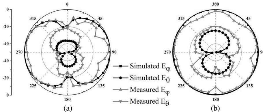
**Figure 10.** Measured and simulated radiation patterns at 2.45 GHz.
