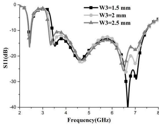
**Figure 6.** Return loss against frequency with different  $W_3$ .
