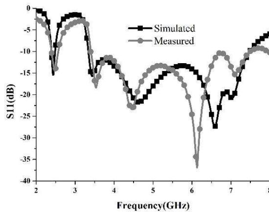
**Figure 9.** Measured and simulated  $S_{11}$  of the proposed antenna.
