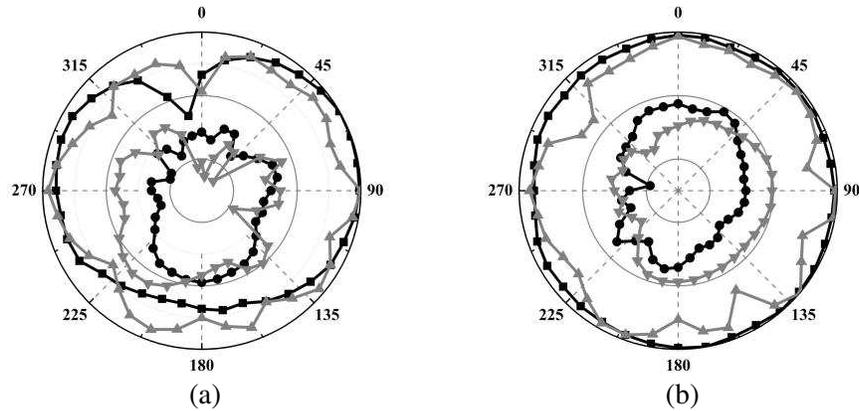
**Figure 12.** Measured and simulated radiation patterns at 5.5 GHz band.
