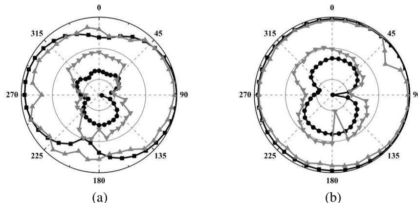
**Figure 11.** Measured and simulated radiation patterns at 3.5 GHz band.
