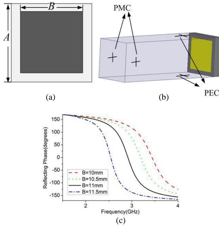
Figure 3. (a) The dimensions of AMC unit. (b) The simulation setup in HFSS. (c) The simulated reflecting phases of the AMC unit with different  $B$ .
