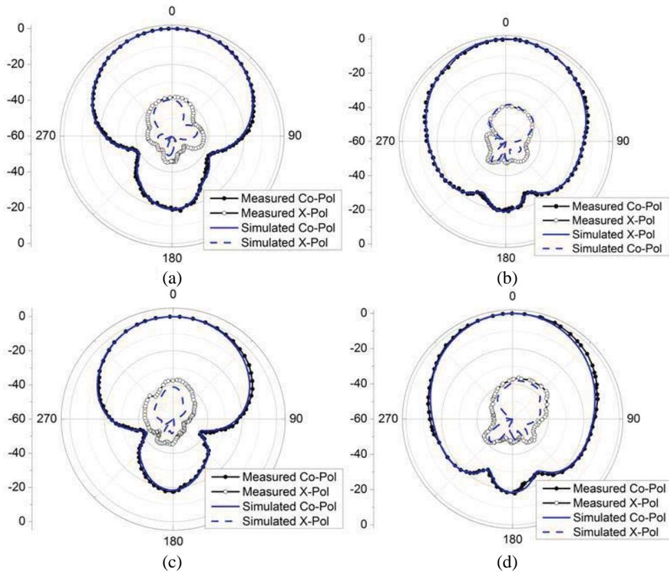
**Figure 5.** Measured and simulated radiation patterns at 2.4 GHz for the proposed antenna. (a) *E*-plane for port 1. (b) *H*-plane for port 1. (c) *E*-plane for port 2. (d) *H*-plane for port 2.
