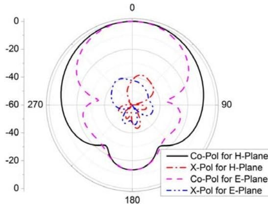
**Figure 6.** Simulated *E*-plane and *H*-plane radiation patterns at 2.4 GHz for the antenna without AMC reflector.
