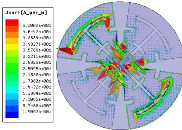
Figure 2. Current distributions of the antenna at 2.4 GHz.
