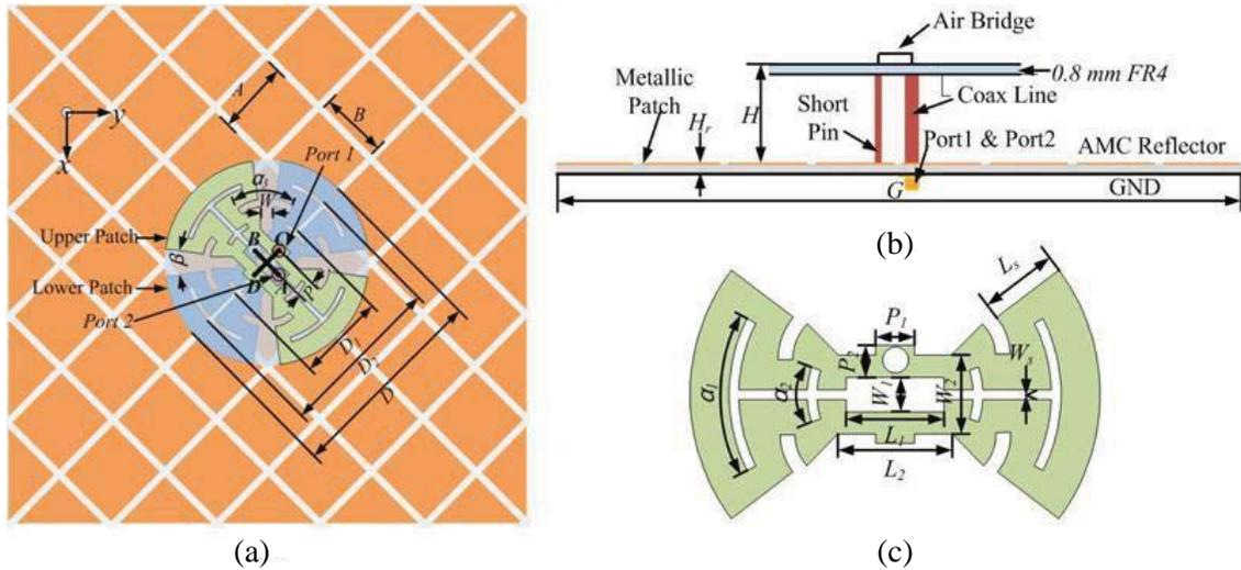
**Figure 1.** Configuration of the proposed dual-polarized patch antenna. (a) The top view. (b) Side view. (c) Dimensions of the circular patch.
