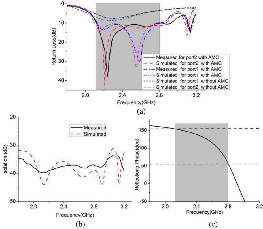
**Figure 4.** (a) Simulated and measured return loss of the proposed antenna. (b) Simulated and measured isolation of the proposed antenna. (c) Simulated reflecting phase of the AMC reflector (Grey area is the operation band of the antenna).
