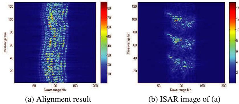
**Figure 2.** Segmented alignment result (3 segment); range profiles are poorly aligned and ISAR is blurred because of the small number of segments.
