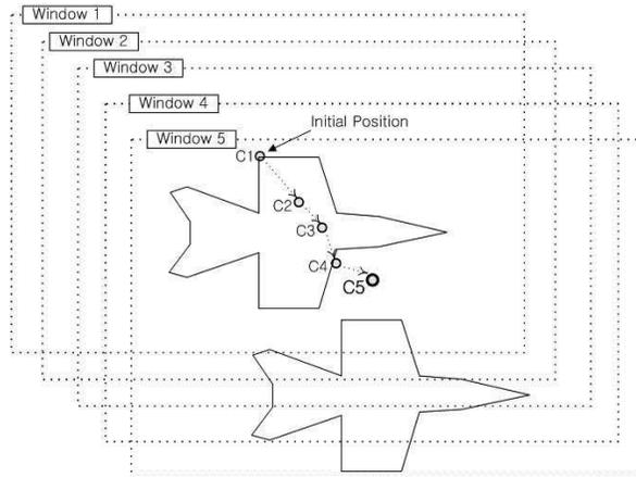
**Figure 3.** Image segmentation using a window larger than twice the target size [10];  $C_n$  = center of mass of window  $n$ . Sums of converted pixel values within windows are compared sequentially until the sum stops increasing. However, each image may not be segmented properly because of the large window size.
