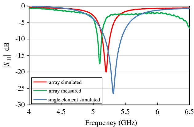
**Figure 4.** Simulated and measured return loss of the proposed antenna.
