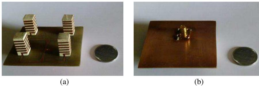
**Figure 3.** Photograph of fabricated antenna, (a) top view, (b) bottom view.
