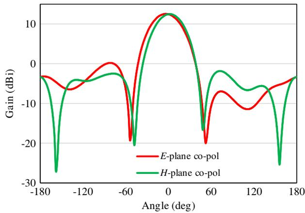
**Figure 6.** Simulated  $E$ -plane and  $H$ -plane radiation pattern of antenna array for the inter-element spacing of 28 mm ( $0.5\lambda$ ).
