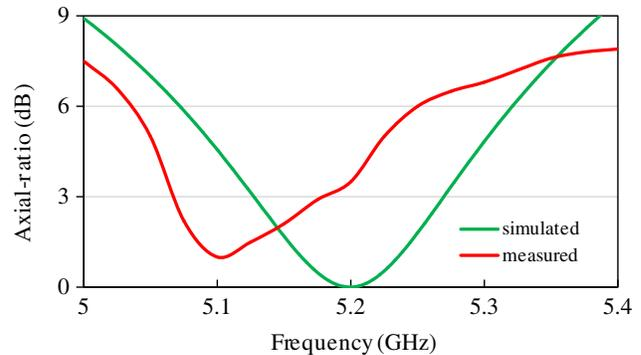
**Figure 11.** Simulated and measured axial-ratio of proposed antenna array.
