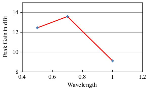
**Figure 10.** Simulated peak gain for different inter-element spacing.
