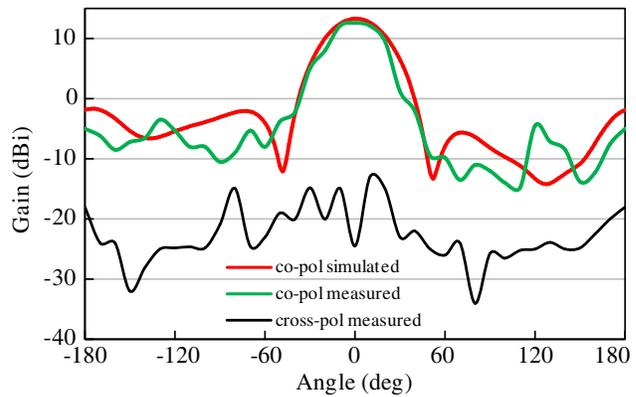
**Figure 9.** Simulated and measured  $H$ -plane radiation pattern of the proposed antenna array.
