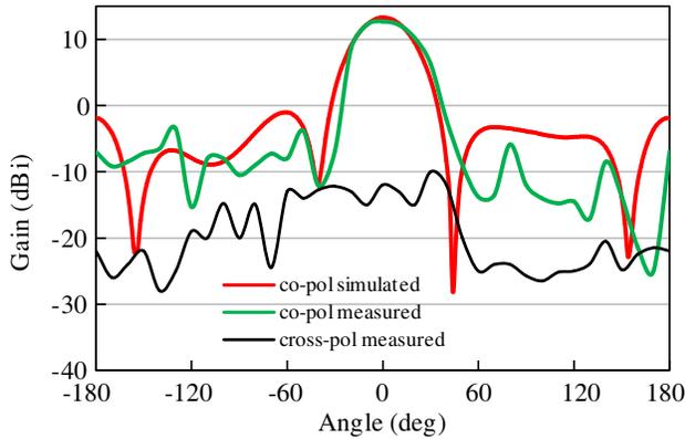
**Figure 8.** Simulated and measured  $E$ -plane radiation pattern of the proposed antenna array.
