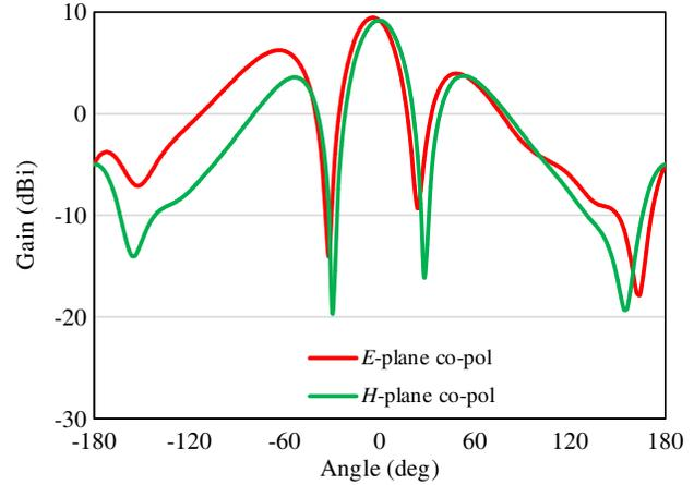
**Figure 7.** Simulated  $E$ -plane and  $H$ -plane radiation pattern of antenna array for the antenna spacing 58 mm ( $1.0\lambda$ ).
