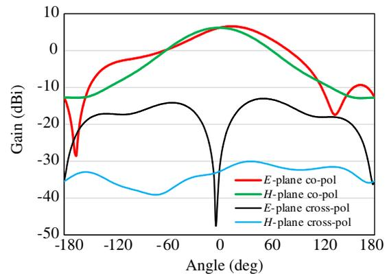
**Figure 5.** Simulated radiation pattern of the single element antenna.
