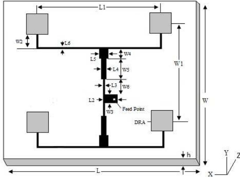
**Figure 1.** Configuration of proposed antenna.
