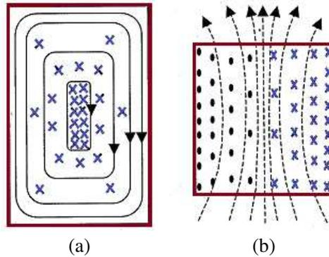
**Figure 2.** Field distribution of  $TE_{\delta 11}$  mode inside a single DRA, (a) electric field in the  $XZ$  plane at  $Y = 0$ , (b) magnetic field in the  $XY$  plane at  $Z = 0$ .
