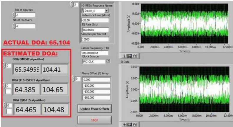
**Figure 17.** Experimental results for two RF sources placed at  $65^\circ$  and  $104^\circ$  from the array reference.
