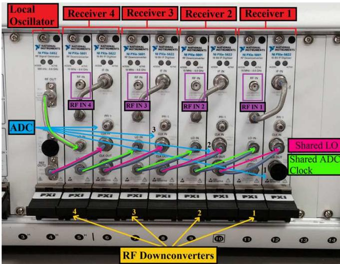
Figure 3. NI-PXI receiver unit.
