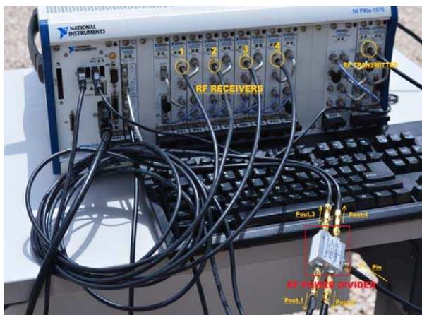
**Figure 7.** Setup for calibrating the phase of the received signals.
