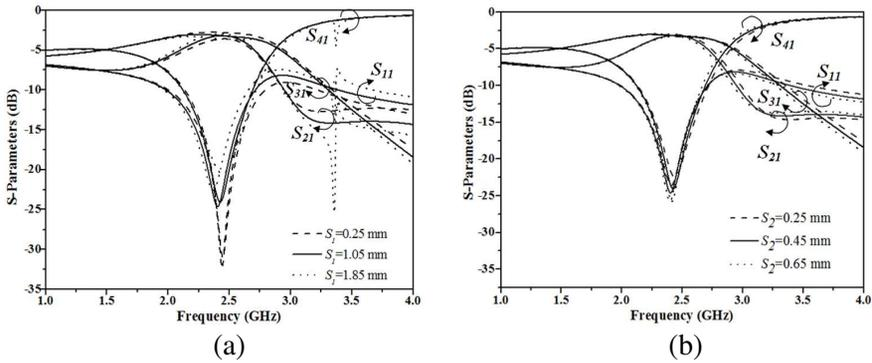
**Figure 3.** Effect on simulated  $s$ -parameters due to variation in (a)  $S_1$ , (b)  $S_2$ .
