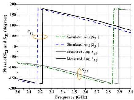
**Figure 7.** Phase of  $S_{21}$  and  $S_{31}$  of the proposed coupler.
