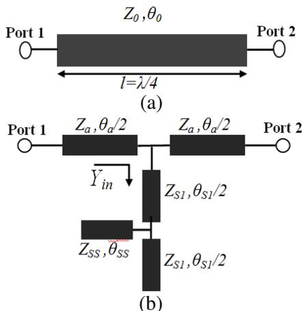
**Figure 1.** (a) Equivalent circuit of quarter wavelength transmission line. (b) Equivalent transmission line model of reduced transmission line using recursively loaded stubs.
