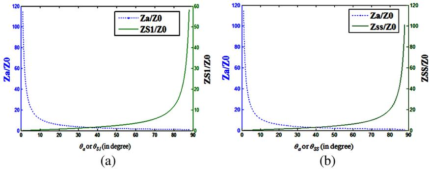
**Figure 2.** (a) Relations between normalized  $Z_a$ , and normalized  $Z_{s1}$  with  $\theta_a$  and  $\theta_{s1}$ . (b) Relations between normalized  $Z_a$ , and normalized  $Z_{ss}$  with  $\theta_a$  and  $\theta_{ss}$ .
