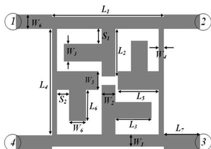
**Figure 4.** Layout of the proposed recursively loaded stub based branch line coupler.
