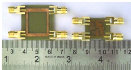
**Figure 5.** Photograph of fabricated prototype of (a) conventional BLC and (b) the proposed recursive stub loaded miniaturized BLC.
