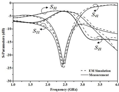
**Figure 6.** Simulated and measured  $S$ -parameters of the proposed BLC.
