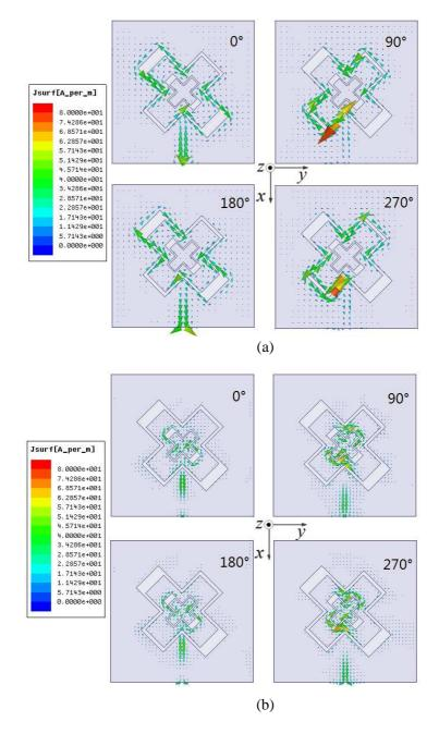
Figure 7. The simulated current distributions at the frequency of (a) 2.45 GHz (b) 5.8 GHz.
