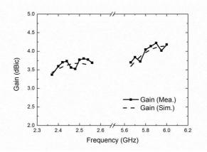
Figure 9. Simulated and measured gain.
