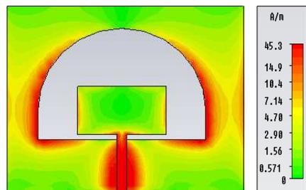
**Figure 8.** Simulated Current distribution of the transparent antenna.
