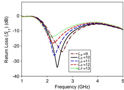
**Figure 6.** Comparison of the simulated return loss for different values of patch length.
