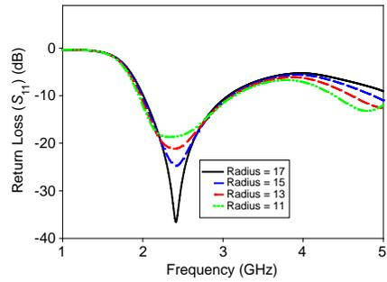
**Figure 4.** Comparison of simulated return loss for different slot radius.
