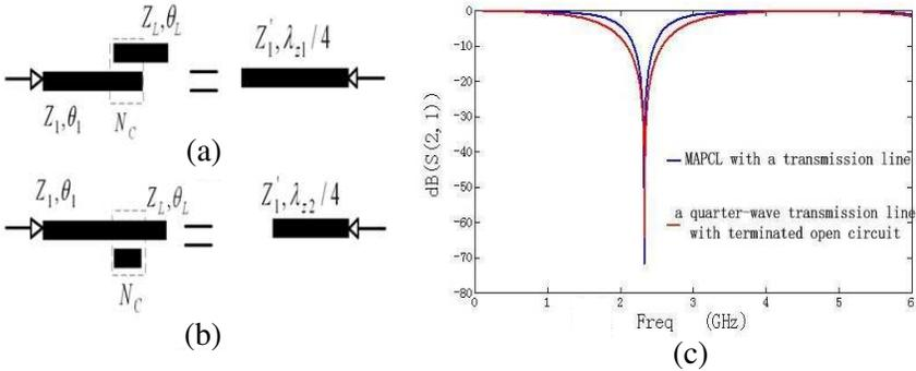
**Figure 5.** Equivalent circuit model: (a) left segment of  $N_D$ , (b) left segment of  $N_U$  and (c) comparison between dB  $|S_{21}|$  of MAPCL with a transmission line and that of a quarter-wave transmission line with terminated open-circuit.
