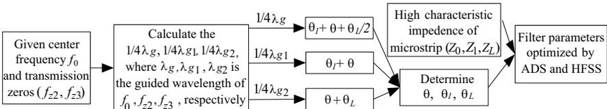
**Figure 6.** Design procedure of the proposed filter.
