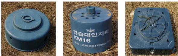
**Figure 10.** The landmines used in the experiments. From the left, each landmine is KM15, KM16 and KM19, respectively.
