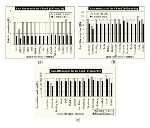
Figure 2. Rain attenuation (dB) in 145 mm/hr. (a) C-band, (b) X-band, (c) Ku-band.
