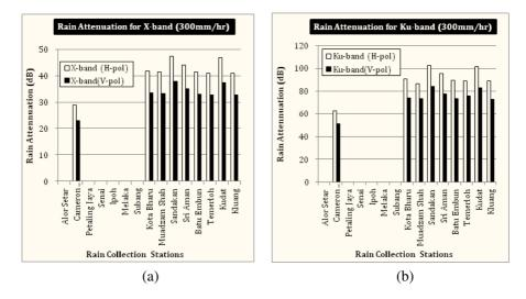
**Figure 4.** Rain attenuation (dB) in 300 mm/hr. (a) X-band, (b) Kuband.
