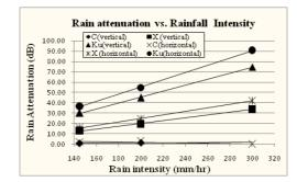
Figure 5. Rain attenuation (dB) versus rainfall density (mm/hr) in the C-, Ku- and X-bands.
