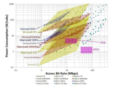
Figure 2. Power consumption per subscriber versus bit rate for mobile WiMAX (black x), LTE (black circle), HSPA (grey +), and LTE Advanced (grey diamond) and femto — (•), micro — (•) and macrocells — (•).
