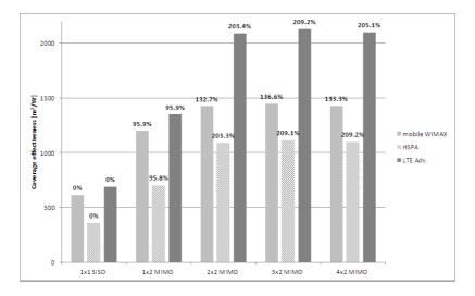
**Figure 4.** Coverage effectiveness and coverage effectiveness gain (in %) for different MIMO systems.
