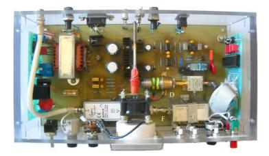
Figure 8. Implementation of the radio telescope. F: bandpass filter; D: detector.
