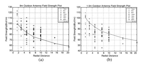
**Figure 6.** Plots of measured field strength and F(50, 90) values for (a) 9 m fixed antenna, (b) 1.5 m portable antenna.
