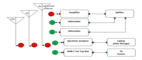
Figure 2. Measurement instrumentation.
