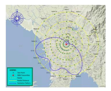
Figure 1. NBN radiation pattern and radial plots.
