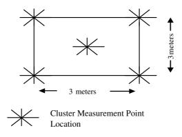
Figure 3. Cluster measurement point arrangements.
