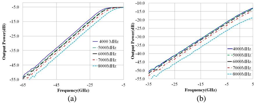
**Figure 3.** Output power vs. available input power (a) for 0 dB attenuation (b) for 31 dB attenuation.
