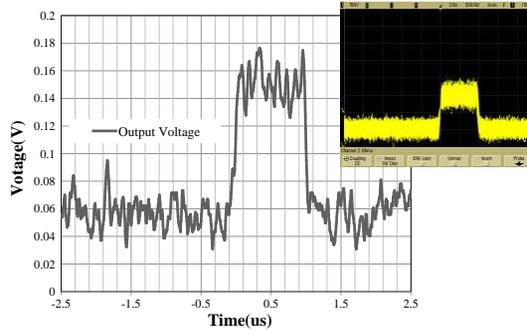
**Figure 4.** Output pulse of DLVA in TSS point.
