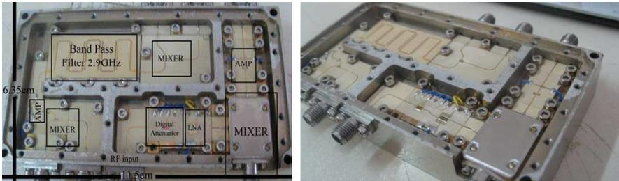
**Figure 8.** Evaluation board for C band down-converter.
