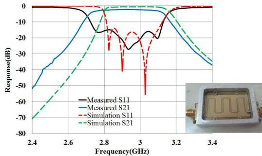
**Figure 6.** Measured and simulation results of 2.9 GHz filter.
