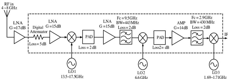
**Figure 1.** Circuit diagram of frequency down-converter.
