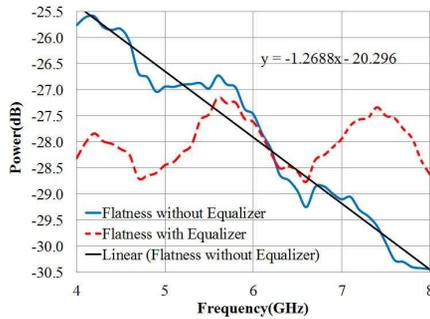
**Figure 7.** Output power vs. input frequency with and without equalizer.
