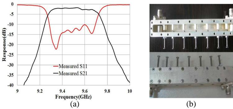
**Figure 5.** (a) Measured results of 9.5 GHz band pass filter. (b) Photograph of the implemented combline filter.
