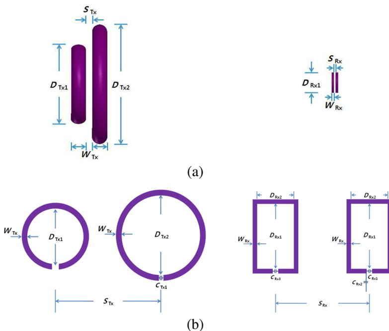
**Figure 12.** Wireless energy transmission resonator consisting of receiving coil with size of iPhone4. (a) Side view. (b) Front view.
