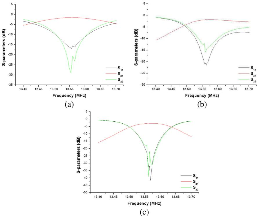
**Figure 10.** Measured  $s$ -parameters of wireless energy transmission resonators having various-sized circular transmitting and receiving coils at transmission distance of 20 cm. (a)  $D_{Tx1} = D_{Tx2} = 40$  cm. (b)  $D_{Tx1} = D_{Tx2} = 20$  cm. (c)  $D_{Tx1} = D_{Tx2} = 10$  cm.
