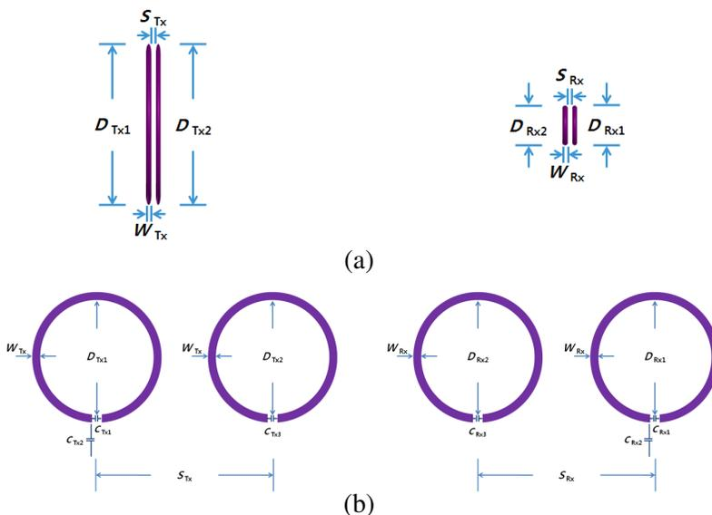
**Figure 8.** Wireless energy transmission resonators having various-sized circular transmitting and receiving coils. (a) Side view. (b) Front view.
