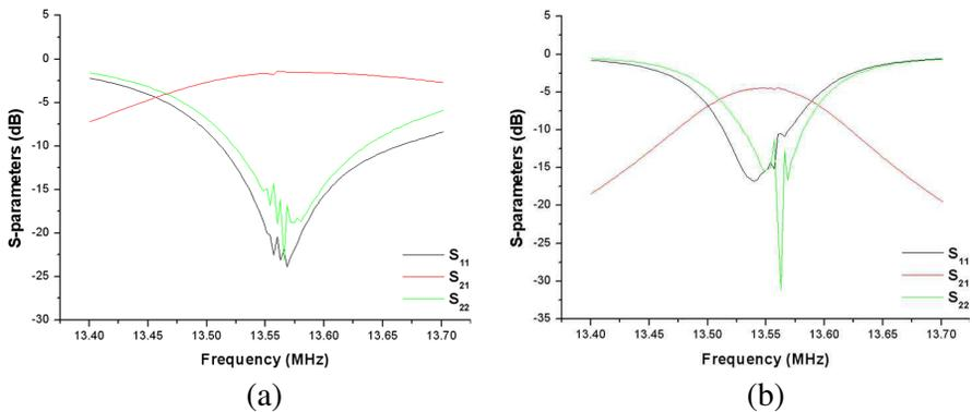
**Figure 14.** Measured  $s$ -parameters of wireless energy transmission resonator consisting of receiving coil with size of iPhone4 at transmission distances of 20 cm and 50 cm. (a) 20 cm. (b) 50 cm.
