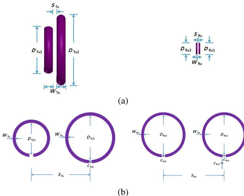
**Figure 1.** Wireless energy transmission resonator having large circular transmitting and small circular receiving coils. (a) Side view. (b) Front view.
