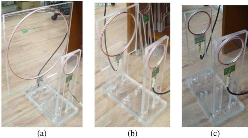
**Figure 9.** Fabrication of wireless energy transmission resonators having various-sized circular transmitting and receiving coils. (a)  $D_{Tx1} = D_{Tx2} = 40\ \text{cm}$ . (b)  $D_{Tx1} = D_{Tx2} = 20\ \text{cm}$ . (c)  $D_{Tx1} = D_{Tx2} = 10\ \text{cm}$ .
