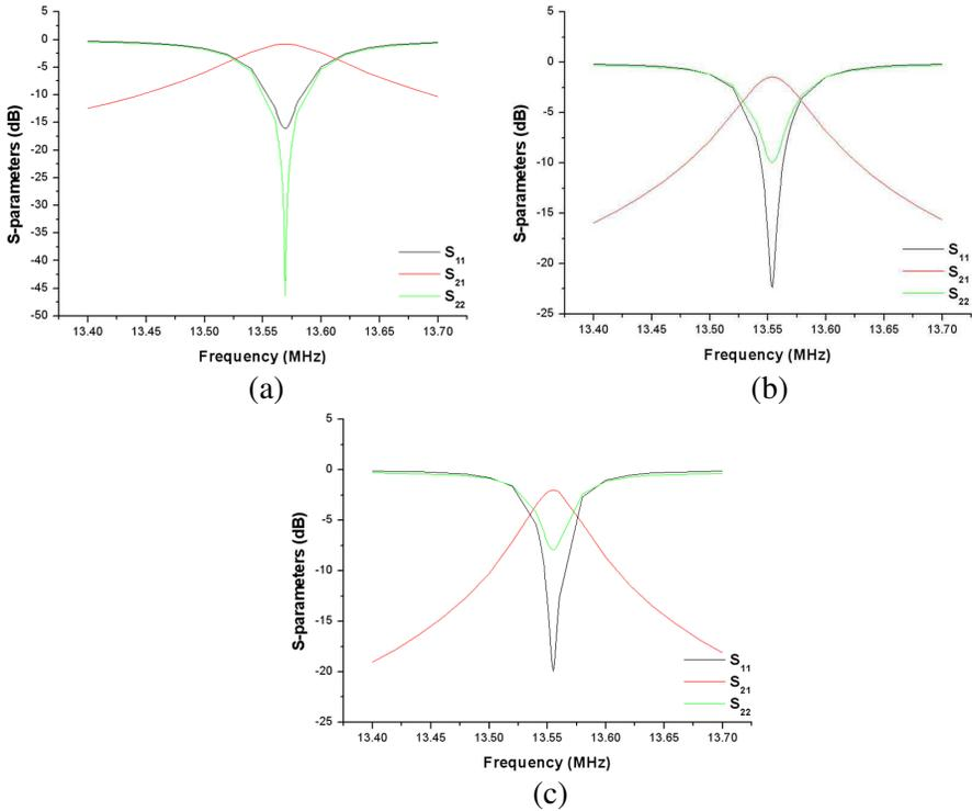
**Figure 2.** Simulated  $s$ -parameters versus transmission distance of wireless energy transmission resonator consisting of large circular transmitting and small circular receiving coils. (a) 20 cm. (b) 30 cm. (c) 40 cm.
