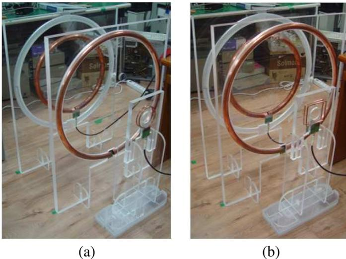
**Figure 5.** Fabrication of wireless energy transmission resonators. (a) Large circular transmitting and small circular receiving coils. (b) Large circular transmitting and small rectangular receiving coils.
