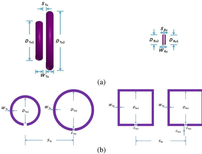
**Figure 3.** Wireless energy transmission resonator having large circular transmitting and small rectangular receiving coils. (a) Side view. (b) Front view.
