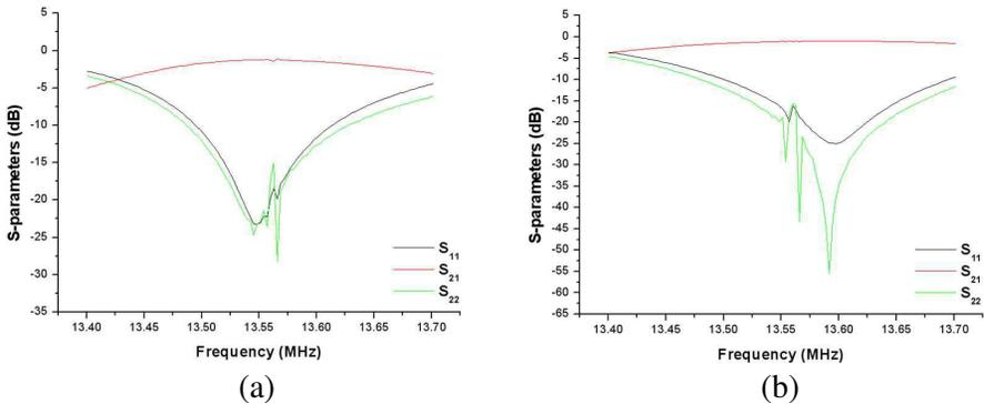
**Figure 6.** Measured  $s$ -parameters of wireless energy transmission resonators at transmission distance of 20 cm. (a) Large circular transmitting and small circular receiving coils. (b) Large circular transmitting and small rectangular receiving coils.
