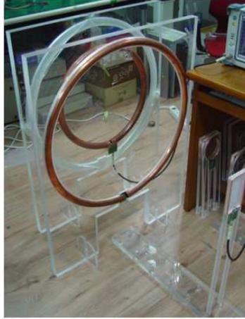
**Figure 13.** Fabrication of wireless energy transmission resonator consisting of the receiving coil with the size of iPhone4.
