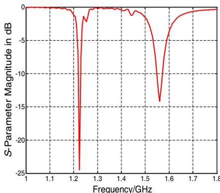
**Figure 5.**  $S$ -parameter performance of our proposed antenna (Figure 1, case 1).  $TM_{010}$  at 1.56 GHz and  $TM_{0\delta 0}$  at 1.224GHz. Radiation performance for both bands are satisfactory.
