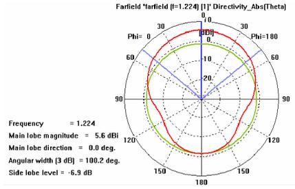
**Figure 7.** Principal *H*-plane radiation pattern (Polar plot) of  $TM_{0\delta 0}$  ( $0 < \delta < 1$ ) of our proposed antenna. Main lobe deviation is  $0^\circ$  from broadside direction.
