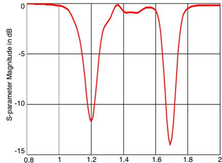
**Figure 12.**  $S$ -parameter performance of our proposed antenna (Figure 1, case 1).  $TM_{010}$  at 1.69 GHz and  $TM_{0\delta 0}$  is at 1.205 GHz.
