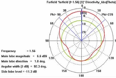
**Figure 8.** Principal *E*-plane radiation pattern (Polar plot) of  $TM_{010}$  of our proposed antenna. Main lobe deviation is only  $1^\circ$  from broadside direction.
