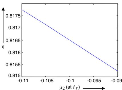
**Figure 3.** The possible choices of filling ratio and corresponding permeability of the MNG metamaterial (at  $f = f_r$ ).
