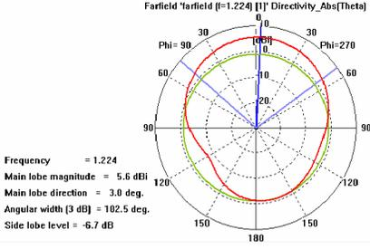
**Figure 6.** Principal *E*-plane radiation pattern (Polar plot) of  $TM_{0\delta 0}$  ( $0 < \delta < 1$ ) of our proposed antenna. Main lobe deviation is only  $3^\circ$  from broadside direction.
