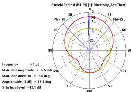
**Figure 16.** Principal *E*-plane radiation pattern (Polar plot) of  $TM_{010}$  of our proposed antenna. Main lobe deviation is only  $2^\circ$  from broadside direction.
