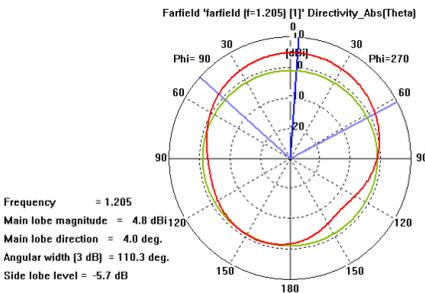
**Figure 14.** Principal  $E$ -plane radiation pattern (Polar plot) of  $TM_{0\delta 0}$  ( $0 < \delta < 1$ ) of our proposed antenna. Main lobe deviation is only  $4^\circ$  from broadside direction.
