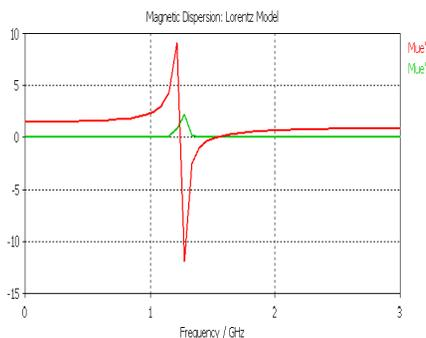
**Figure 4.** Lorentz dispersive model for proposed antenna (design-1).
