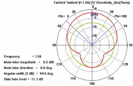
**Figure 9.** Principal *H*-plane radiation pattern (Polar plot) of  $TM_{010}$  of our proposed antenna. Main lobe deviation is  $0^\circ$  from broadside direction.
