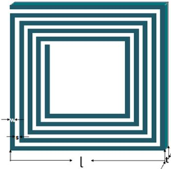
**Figure 11.** Geometrical dimensions of SR:  $w = 0.1$  mm,  $s = 0.1$  mm,  $t = 0.1$  mm,  $l = 4.8$  mm. Number of cells used = 7 in our actual design (Figure 10(a)).
