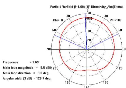
**Figure 17.** Principal *H*-plane radiation pattern (Polar plot) of  $TM_{010}$  of our proposed antenna. Main lobe deviation is  $3^\circ$  from broadside direction.
