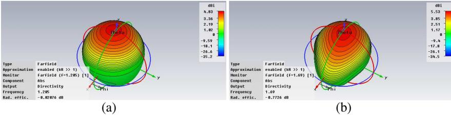
**Figure 13.** Three dimensional radiation pattern of (a)  $TM_{0\delta 0}$  mode at 1.205 GHz and (b)  $TM_{010}$  mode at 1.69 GHz. Directivities are quite satisfactory.
