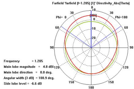
**Figure 15.** Principal  $H$ -plane radiation pattern (Polar plot) of  $TM_{0\delta 0}$  ( $0 < \delta < 1$ ) of our proposed antenna. Main lobe deviation is  $0^\circ$  from broadside direction.
