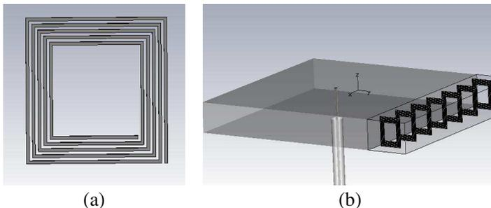
**Figure 10.** (a) Actual Spiral Resonator used in our design (Dimension details are given in Figure 11). (b) Implementation of SR arrays underneath the patch to obtain MNG behavior at the desired frequency for  $50 \text{ mm} \times 40 \text{ mm}$  antenna (Figure 1, case 1).
