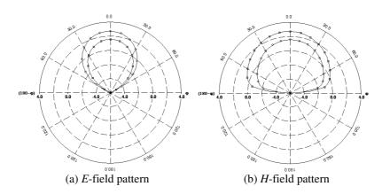
Figure 10. Simulated radiation pattern at 3.4 GHz.
