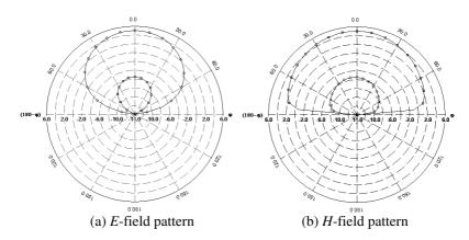
Figure 11. Simulated radiation pattern at 3. 45 GHz.
