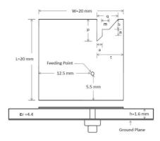
Figure 1. Antenna 1 configuration.
