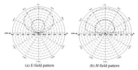
Figure 9. Simulated radiation pattern at 3.345 GHz.
