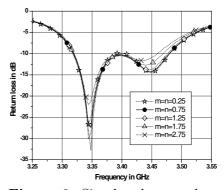
Figure 8. Simulated return loss for different values of 'm' and 'n' on the 1st band.
