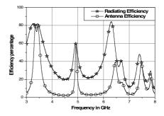
Figure 13. Efficiency versus frequency plot for the antenna 2.
