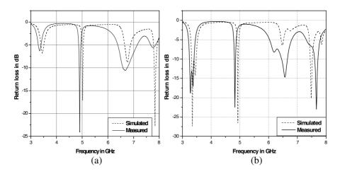
Figure 18. Comparison between measured and simulated return losses (a) antenna 1, (b) antenna 2.
