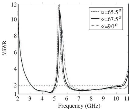
**Figure 2.** Simulated VSWR of the proposed UWB BNCS antenna as a function of *annular sector* ( $\alpha$ ).
