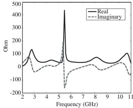
**Figure 7.** Calculated input impedance of the proposed UWB BNCS antenna.
