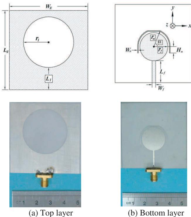
**Figure 1.** Geometry and photograph of the proposed UWB BCNS antenna; (a) Circular slot. (b) Feed network with parasitic strip.
