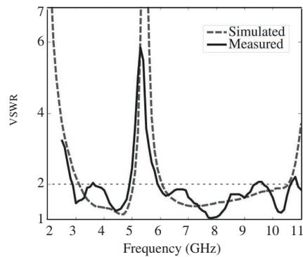
**Figure 5.** Simulated and measured VSWR of the proposed UWB BNCS antenna with dimensions of Table 1.
