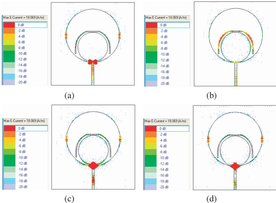
**Figure 6.** Simulated current distribution of the proposed UWB BNCS antenna at frequencies: (a) 4 GHz, (b) 5.15 GHz, (c) 8 GHz, and (d) 10 GHz.
