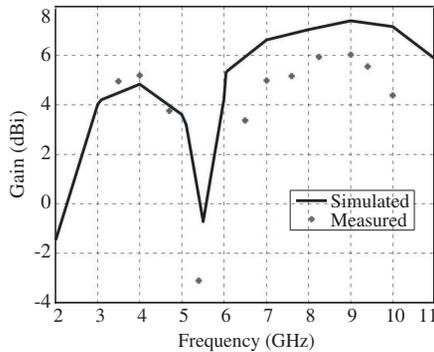
**Figure 9.** Simulated and measured gain of the proposed UWB BNCS antenna.
