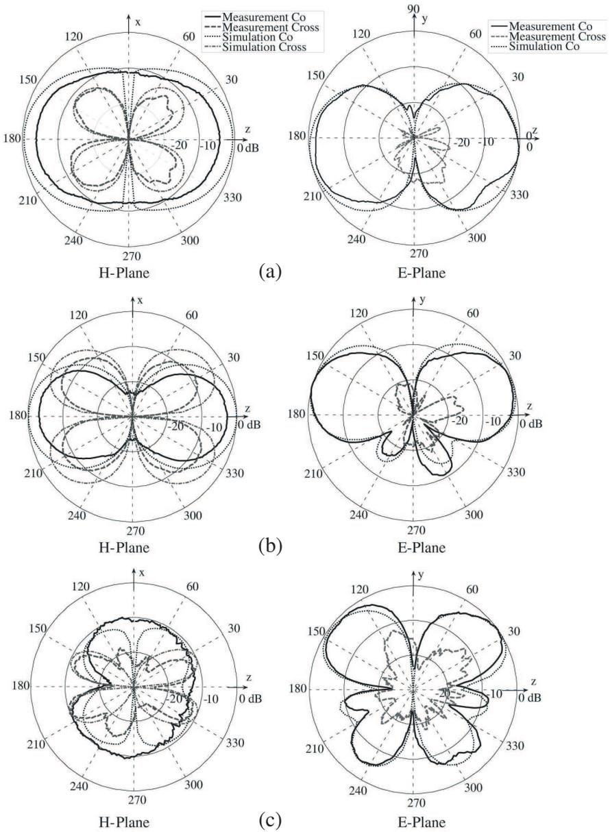
**Figure 8.** Simulated and measured radiation patterns of the UWB BNCS proposed antenna at frequencies: (a) 4 GHz, (b) 7 GHz, (c) 10 GHz.
