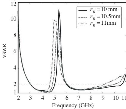
**Figure 4.** Simulated VSWR of the proposed UWB BNCS antenna as a function of *inner radius of the annular strip* ( $r_n$ ).
