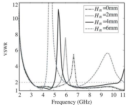
**Figure 3.** Simulated VSWR of the proposed UWB BNCS antenna as a function of  $H_n$ .
